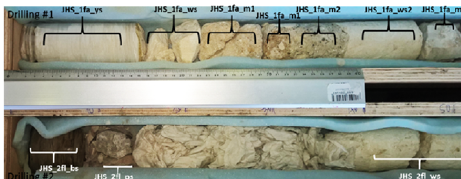
Figure 10 Above: Façade core sample: Three building stones samples (JHS_1fa_ys, JHS_1fa_ws, JHS_1fa_ws2), Three mortar samples (JHS_1fa_m1, JHS_1fa_m2, JHS_1fa_m3) Below: Floor core sample: Three building stones samples (JHS_2fl_bs, JHS_2fl_ps, JHS_2fl_ws)
