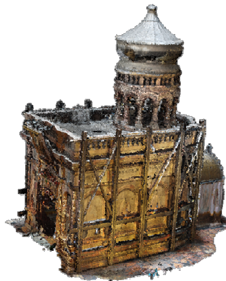
Figure 16 The colored point cloud of the Holy Aedicule
