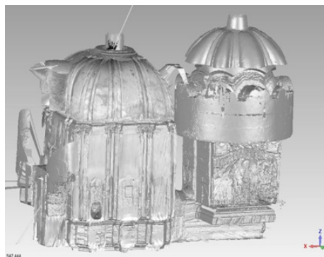
Figure 18 Part of the registered point clouds inside the Holy Aedicule
