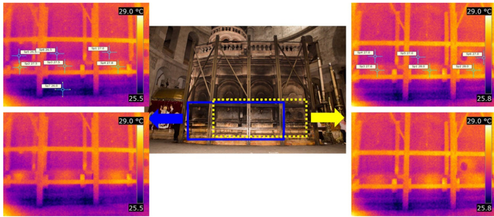
Figure 11 IR-Thermal inspection of the south façade of the Holy Aedicule of the Church of the Holy Sepulchre
