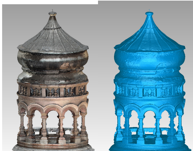
Figure 17 The 3D model of the dome textured (left) and non-textured (right)
