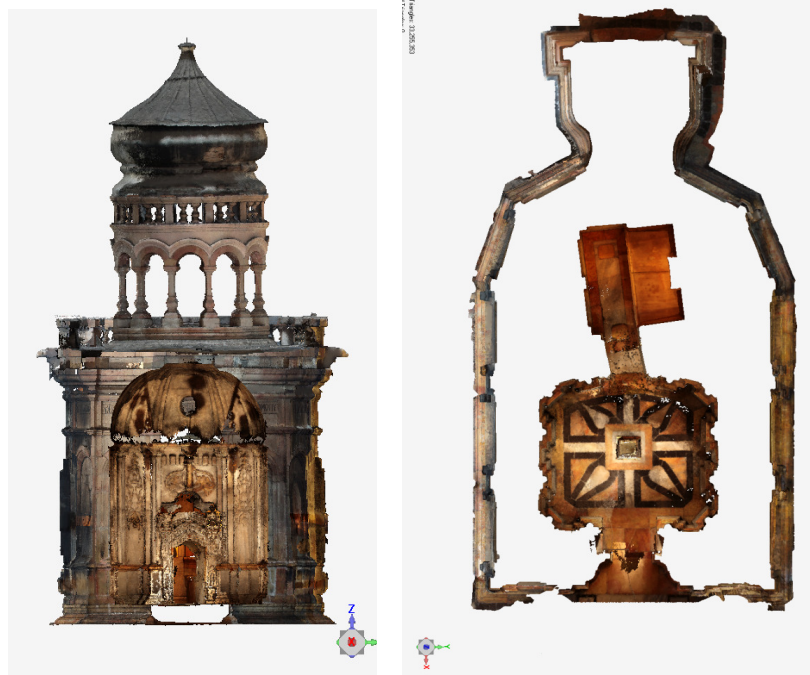
Figure 21 Left: Visualization of a vertical section from the 3D model with texture Right: Horizontal section of the 3D model where the floor is shown
