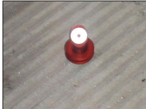
Photo 8: The magnetic target.
