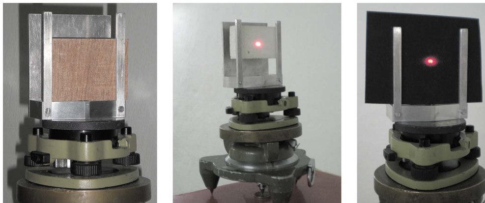
Fig. 5. Reflectorless measurement on marble, black paper, and wood
