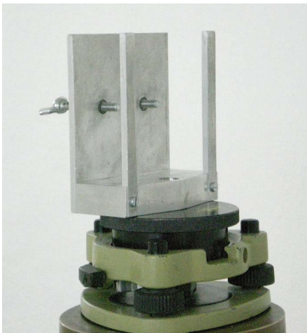
Fig. 2. Special base for supporting the target materials
