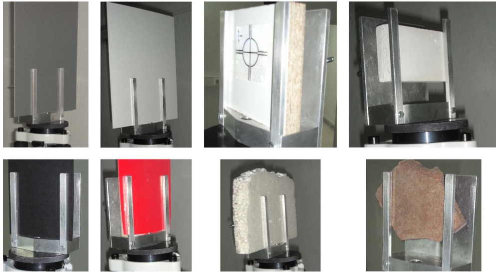
Fig. 1. Some of the materials: (a) Kodak gray card; (b) Kodak white card; (c) reflective tape target; (d) white cement; (e) black paper; (f) red plastic; (g) white foam; and (h) roof tile
