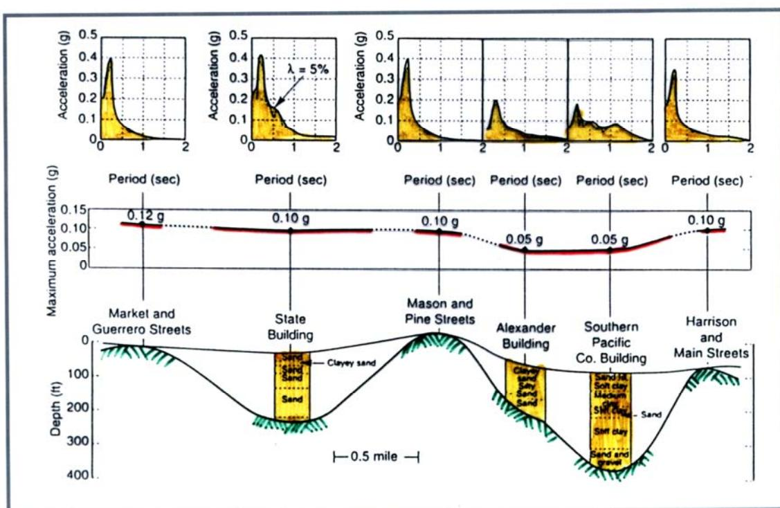
Variation of peak ground acceleration and elastic response spectra in connection with local soil conditions at recording stations . . .
