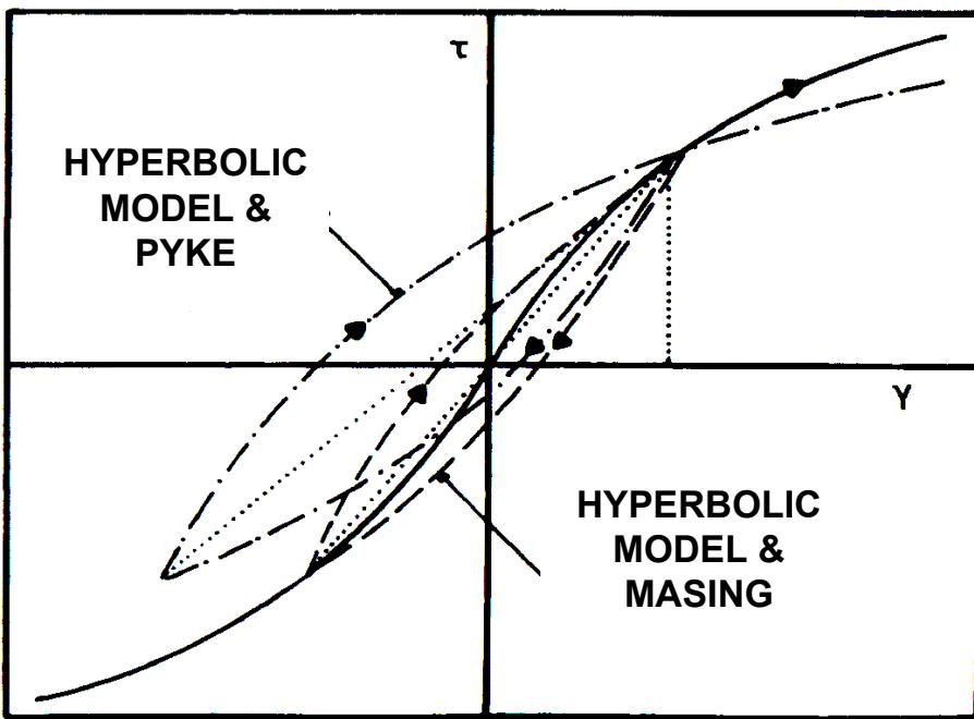
**Cyclic unloading - reloading according to PYKE (1979)**
