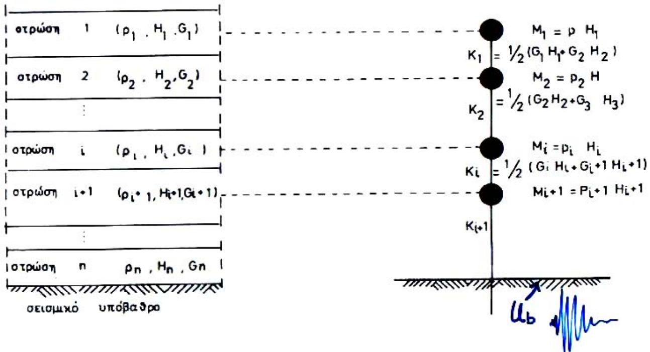
The layered soil profile is discretized and simulated as a system of lumped masses and visco-elastic springs . . .
