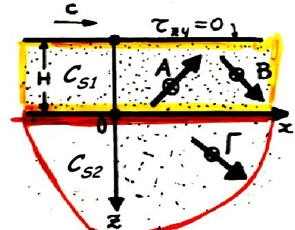
$$\begin{Bmatrix} A e^{-i r_1 k_H} - B e^{i r_1 k_H} = 0 \\ A + B - \Gamma = 0 \\ A(G_1 r_1) + B(G_1 r_1) - \Gamma(G_2 r_2) = 0 \end{Bmatrix} \text{ substituting for } A, B, \Gamma \text{ gives:}$$
