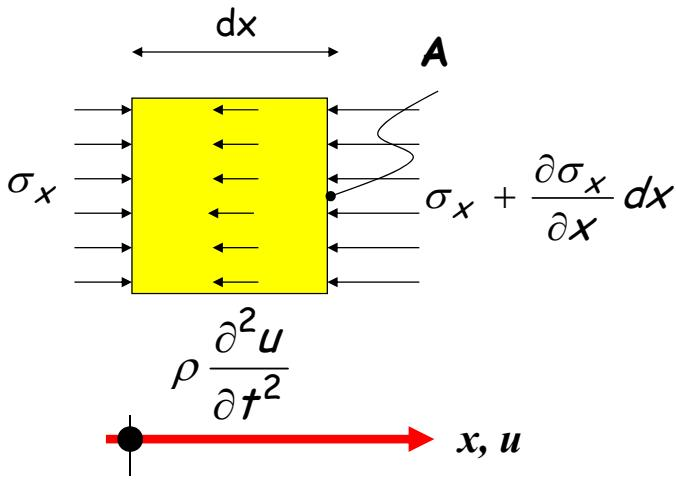
$$\sigma_x A = \left( \sigma_x + \frac{\partial \sigma_x}{\partial x} dx \right) A + \rho \frac{\partial^2 u}{\partial t^2} dV$$
