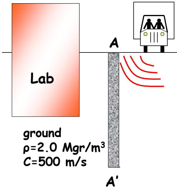
To isolate a precision measurement laboratory (e.g. a geotech lab.) from traffic vibrations, it is proposed to construct the trench AA'. Which of the following two fill materials is preferable :
