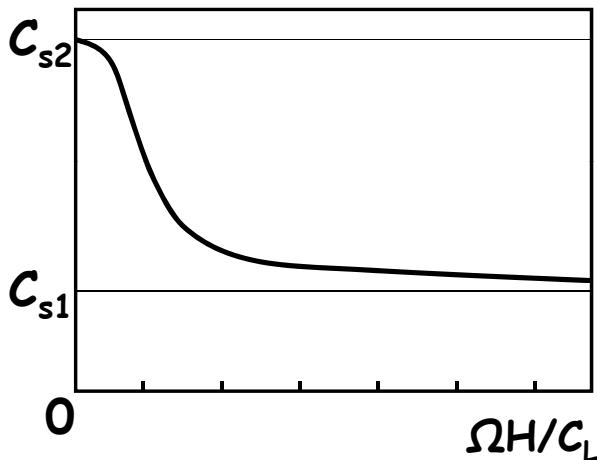
$$\tan \left[ \frac{\omega H}{C_L} \sqrt{\frac{C_L^2}{C_{S1}^2} - 1} \right] = - \frac{G_2}{G_1} \frac{\sqrt{1 - \frac{C_L^2}{C_{S2}^2}}}{\sqrt{\frac{C_L^2}{C_{S1}^2} - 1}}$$
