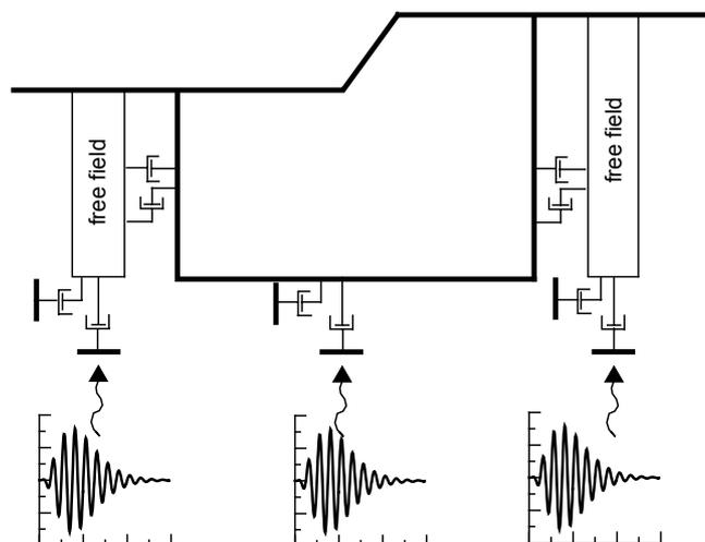
Fig. 1: Schematic illustration of finite difference model for step-like surface topography, the applied boundary conditions and examples for the incoming Chang's signal – type time histories
