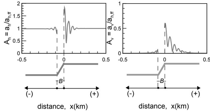
Fig. 3: Typical results for the topographic amplification of the peak horizontal  $A_h$  and the parasitic vertical  $A_v$  acceleration, as a function of horizontal distance  $x$  from the crest (results for  $H/\lambda=2$ ,  $i=30^\circ$ ,  $N=6$ ,  $\xi=5\%$ )
