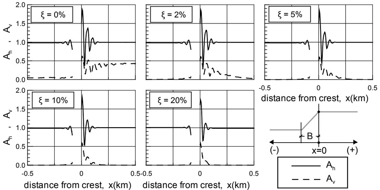
Fig. 8: Effect of number of soil damping  $\zeta$  on the amplification of peak horizontal  $A_h$  and parasitic vertical  $A_v$  acceleration, as a function of distance  $x$  from the crest of a step-like slope (results for  $H/\lambda = 2$ ,  $i = 30^\circ$  and  $N = 4$ )
