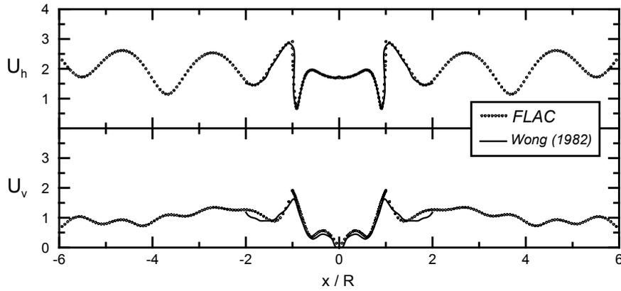
Fig. 2: Analytical verification of numerical scheme for canyon topography (for vertical SV wave,  $R=25\text{m}$ ,  $\lambda/R=2$ )
