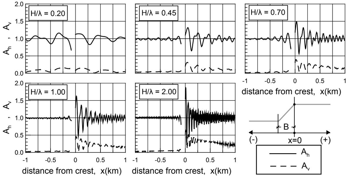
Fig. 6: Effect of normalized height  $H/\lambda$  on the amplification of peak horizontal  $A_h$  and parasitic vertical  $A_v$  acceleration, as a function of distance  $x$  from the crest of a step-like slope (results for  $i=30^\circ$ , harmonic motion,  $\zeta < 5\%$ )
