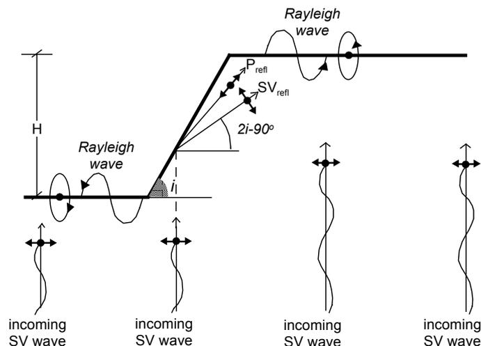
Fig. 4: Schematic illustration of incoming SV waves and induced  $P_{\text{refl}}$ ,  $SV_{\text{refl}}$  and Rayleigh in the case of steep step-like slopes ( $i \geq 45^\circ$ )
