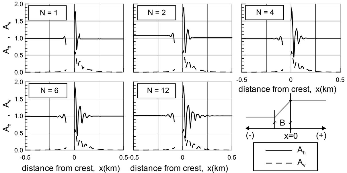
Fig. 7: Effect of number of significant cycles  $N$  on the amplification of peak horizontal  $A_h$  and parasitic vertical  $A_v$  acceleration, as a function of distance  $x$  from the crest of a step-like slope (results for  $H/\lambda = 2$ ,  $i=30^\circ$  and  $\zeta = 5\%$ )
