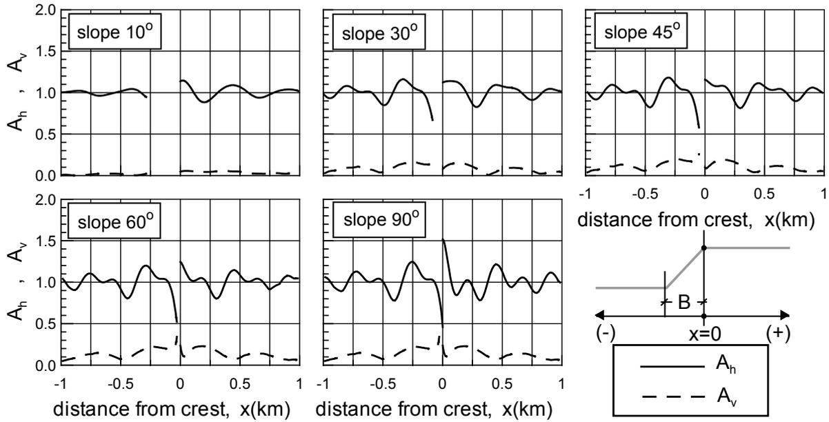
Fig. 5: Effect of slope inclination  $i$  on the amplification of peak horizontal  $A_h$  and parasitic vertical  $A_v$  acceleration, as a function of distance  $x$  from the crest of a step-like slope (results for  $H/\lambda = 0.2$ , harmonic motion and  $\zeta < 5\%$ )
