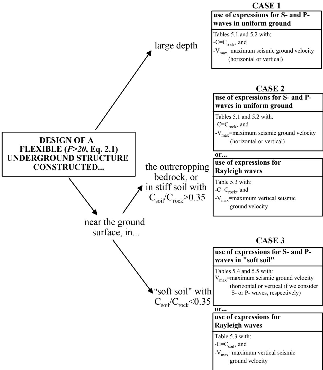
**Figure 2.** Flow chart for the calculation of design strains in underground structures due to seismic wave propagation.
