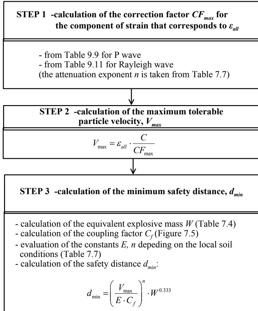
**Figure 5.** Flow chart for the design of underground structures against blasts-Case B: Calculation of the minimum safety distance from a potential blast source.
