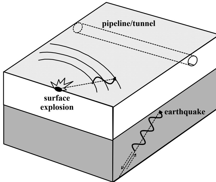
**Figure 1.** Propagation of ground shock waves provoked by an earthquake or a ground surface explosion.
