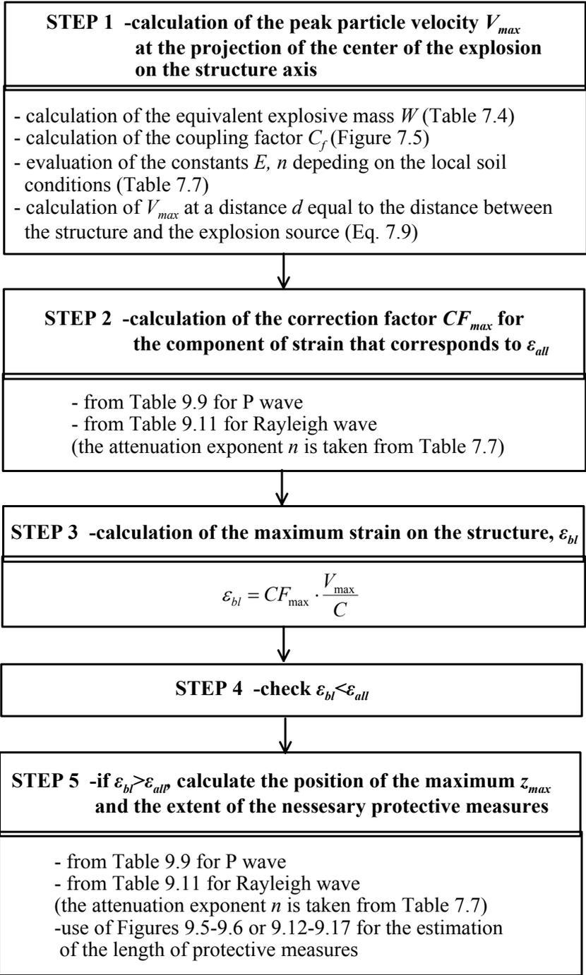
**Figure 4.** Flow chart for the design of underground structures against blasts-Case A: Comparison of the dynamic strain with the maximum allowable strain, for a given distance of the structure from the blast source.
