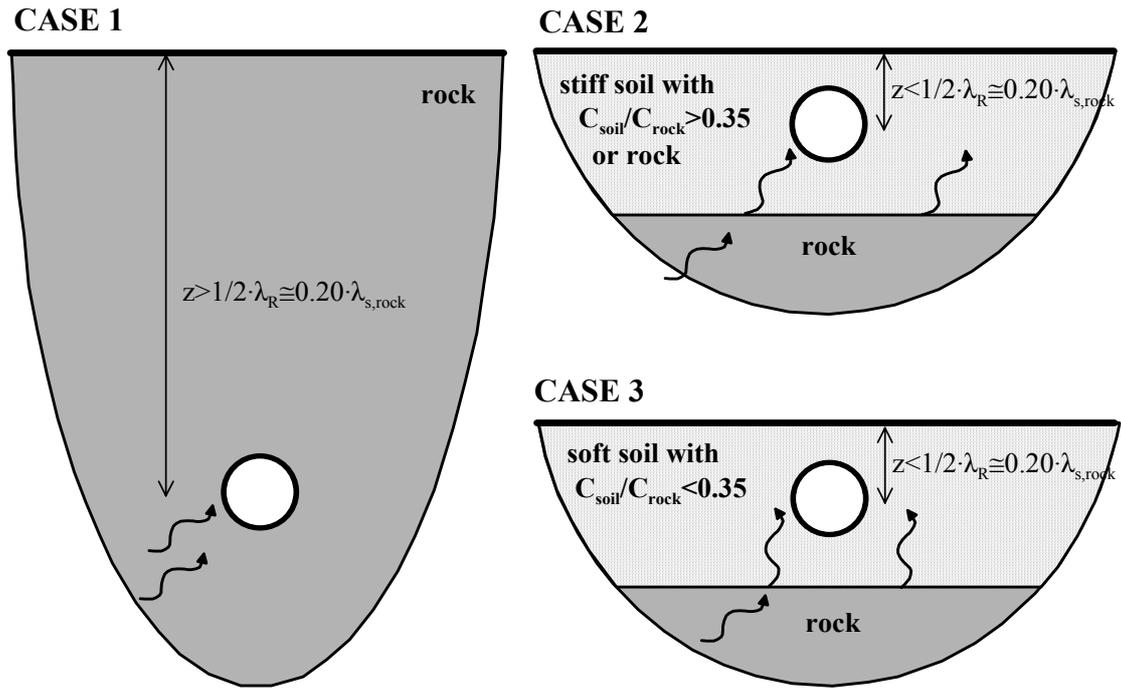
**Figure 3.** Classification of underground structures with respect to the local soil conditions and the depth of construction.
