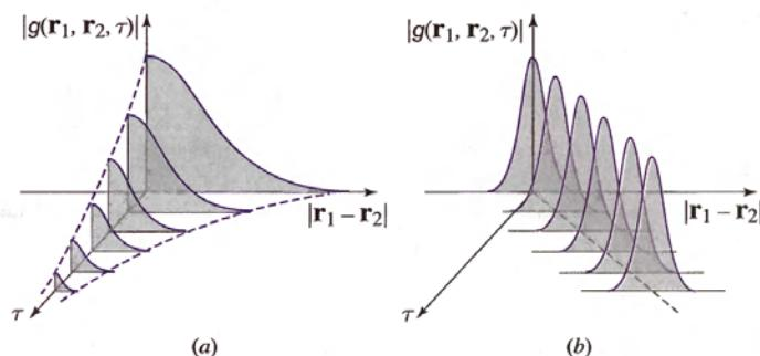
**Figure 11.1-7** Two examples of  $|g(\mathbf{r}_1, \mathbf{r}_2, \tau)|$  as a function of the separation  $|\mathbf{r}_1 - \mathbf{r}_2|$  and the time delay  $\tau$ . In (a) the maximum correlation for a given  $|\mathbf{r}_1 - \mathbf{r}_2|$  occurs at  $\tau = 0$ . In (b) the maximum correlation occurs at  $|\mathbf{r}_1 - \mathbf{r}_2| = c\tau$ .
