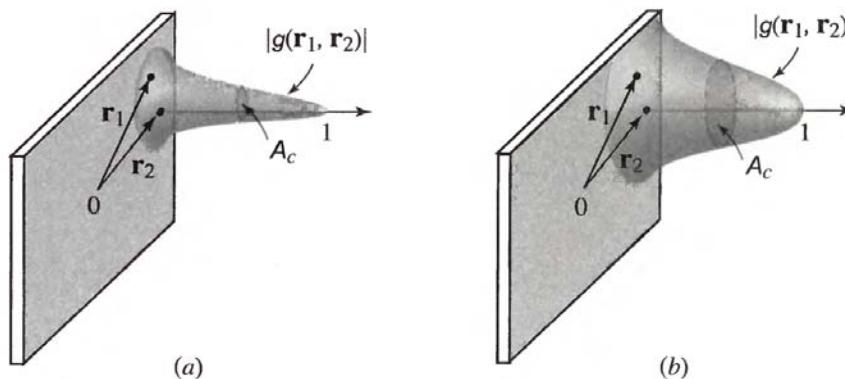
**Figure 11.1-8** Two illustrative examples of the magnitude of the normalized mutual intensity as a function of  $\mathbf{r}_1$  in the vicinity of a fixed point  $\mathbf{r}_2$ . The coherence area in (a) is smaller than that in (b).
