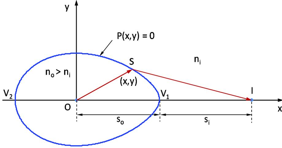
**Figure 5:** A Cartesian ovoid of refractive index  $n_o$  is shown in a surrounding medium of refractive index  $n_i$ . The shape shown is valid for  $n_o > n_i$ . Every ray from the point object  $O$  ends up in the image point  $I$ . The function of the ovoid is  $P(x, y) = 0$ . The distances  $s_o$  and  $s_i$  are the object and image distances from the ovoid's left vertex.
