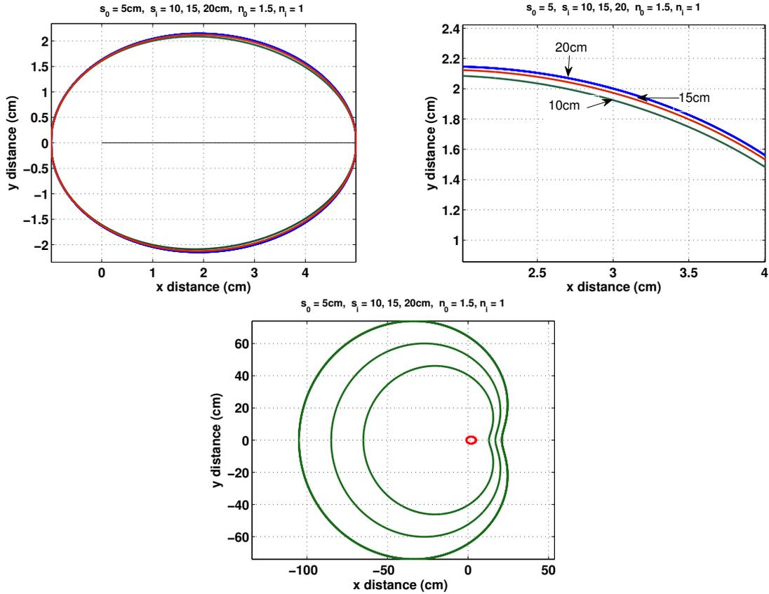
**Figure 6:** Cartesian ovoids for the case of  $n_o > n_i$ . These are the ovoids for  $n_o = 1.5$ ,  $n_i = 1.0$ ,  $s_o = 5 \text{ cm}$ , and  $s_i = 10, 15, 20 \text{ cm}$ . The useful ovoids are the egg-like ones that are very similar since the points  $V_1$  and  $V_2$  do not depend on  $s_i$ .
