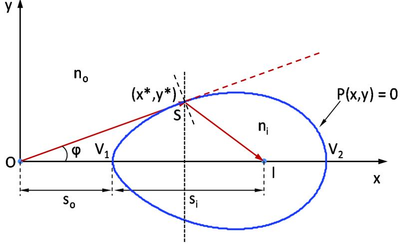
**Figure 3:** The same Cartesian ovoid with the incident from  $O$  beam being tangential to the ovoid. This specifies the maximum angle  $\phi$  that by refraction should pass from point  $I$ . The  $(x^*, y^*)$  denotes the point on the ovoid that the beam is tangential.
