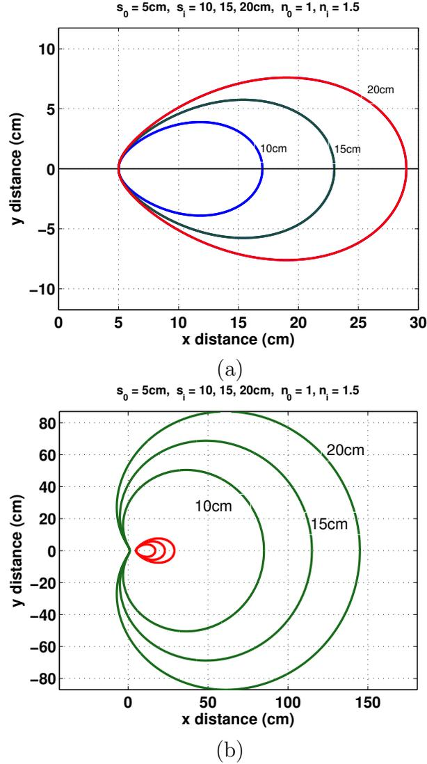
**Figure 2:** The three generated Cartesian ovoids are shown for the parameters  $n_o = 1.0$ ,  $n_i = 1.5$ ,  $s_o = 5$  cm and  $s_i = 10, 15$ , and  $20$  cm. Just for information the other solution that corresponds to the larger root of Eq. (5) is also shown in Fig. 2b along with the smaller solutions in the same scale. The second (larger) solution is not accepted from a physical point of view. These ovoids are known in the literature as Cartesian ovoids.
