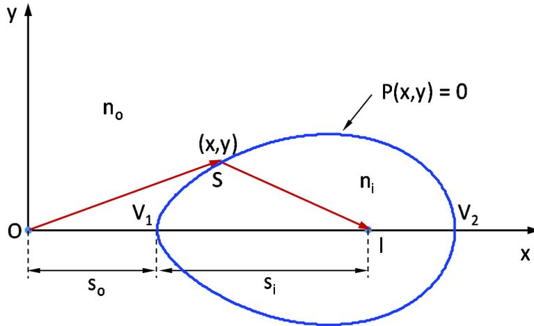
**Figure 1:** A Cartesian ovoid of refractive index  $n_i$  is shown in a surrounding medium of refractive index  $n_o$ . The shape shown is valid for  $n_o < n_i$ . Every ray from the point object  $O$  ends up in the image point  $I$ . The function of the ovoid is  $P(x, y) = 0$ . The distances  $s_o$  and  $s_i$  are the object and image distances from the ovoid's left vertex.
