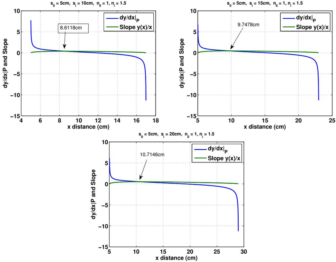
**Figure 4:** Graphical solution for determining the point for which the incident beam from  $O$  is tangential to the ovoid. The intersection of the two curves gives the point  $x^*$  and then  $y^*$  can be determined from the equation of the ovoid  $P(x^*, y^*) = 0$ .
