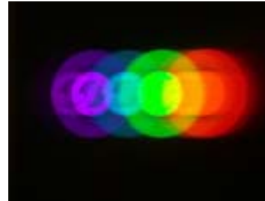
Compact Fluorescent Bulb Emission Spectrum
