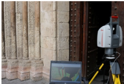
Figure 2: HDS ScanStation 2 during the data acquisition
