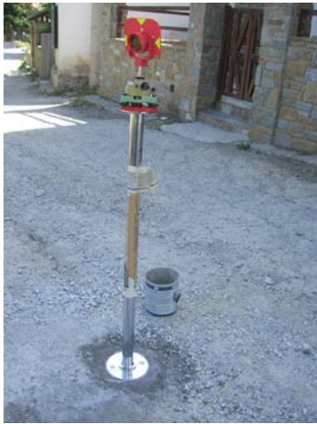
Figure 4: Special markers for the network points
