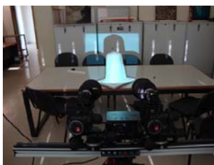
Figure 8. XYZRGB structured light scanner setup for the acquisition of data for the plaster model
