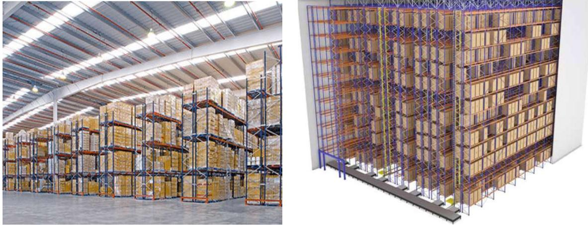
**Figure 1-6:** Examples of existing storage warehouses: **a)** Traditional pallet racking system, height 8 m; **b)** ARSW, height 35<sup>3</sup>
