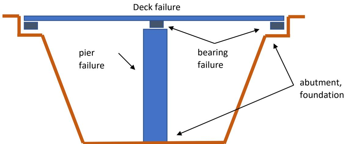
Figure 4. Conceptual breakdown of bridge to components and associated fragilities
