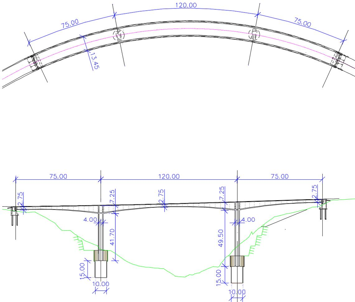
Figure 1. Plan (top) and longitudinal (bottom) section of the G7 bridge, Egnatia Odos, Metsovo (dimensions in meters).
