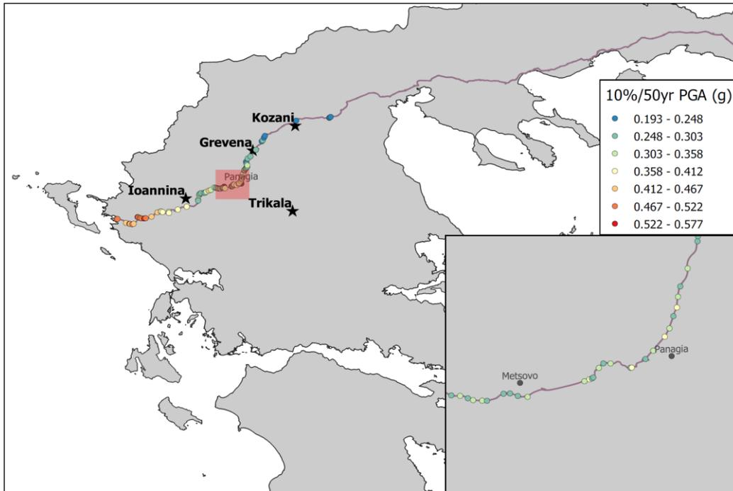
Figure 5. Spatial nature of seismic hazard along a continuous part of the Egnatia Odos highway: 10% in 50yrs PGA values according to the SHARE model (Giardini et al. 2013). The insert figure in the bottom right shows the area of interest for the pilot study (Metsovo-Panagia).
