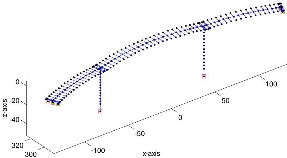
Figure 3. Opensees reduced-order model of the G7 bridge, Egnatia Odos, Metsovo (dimensions in meters). Dummy nodes and elements have been added left and right of the centreline deck elements to visualize the deck width.
