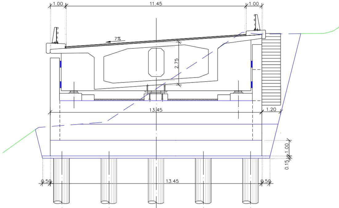
Figure 2: Abutment – bridge connection details (dimensions in meters).
