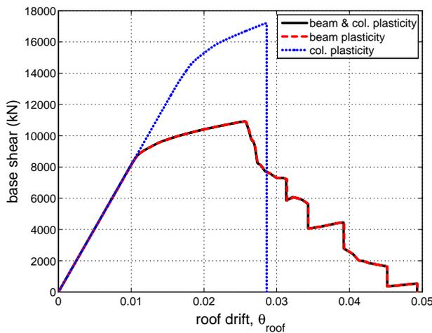
Figure 2: First-mode pushover curves for the BCP, BP, and CP mean parameter models; note that ignoring column plasticity for the BP model does not reduce its accuracy.
