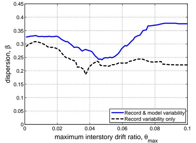
Figure 7:  $S_a$  capacity dispersion for the CP model, showing a significant increase due to parameter uncertainties for drifts higher than 4.5%.
