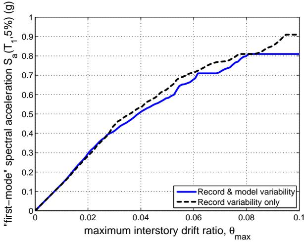
Figure 4: The median IDA curves for the BP model. Plastic hinge uncertainty slightly lowers the median curve, increasing demand and reducing capacity.
