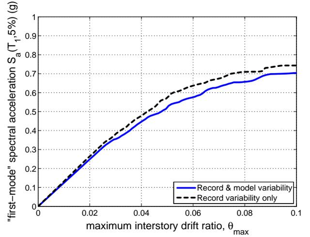
Figure 5: The median IDA curves for the CP model. Plastic hinge uncertainty has a small detrimental effect on the central values of response or capacity.
