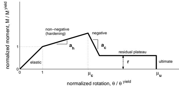
Figure 3: The moment-rotation backbone used for beam and column point hinges shown with its six controlling parameters.
