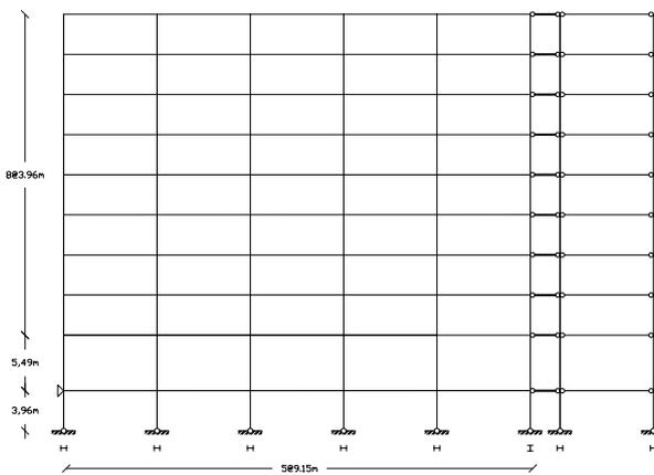
Figure 1: Structural model of the 9-story steel frame, including 5 moment-resisting bays and a single gravity-framing bay on the right instead of the typical leaning column.
