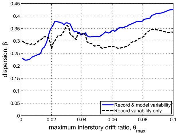
Figure 6:  $S_a$  capacity dispersion for the BP model, showing a moderate increase due to parameter uncertainties for drifts higher than 5%.
