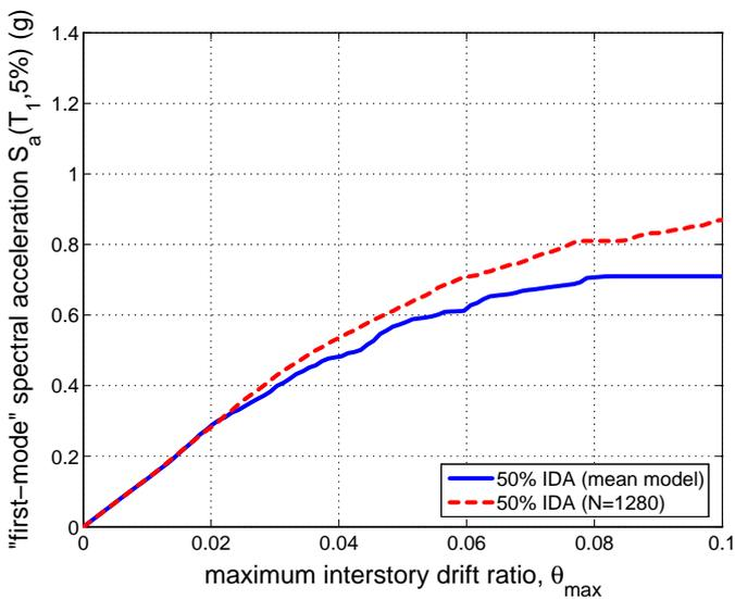
Figure 6: Comparison of median IDAs: iLHS versus the mean model.
