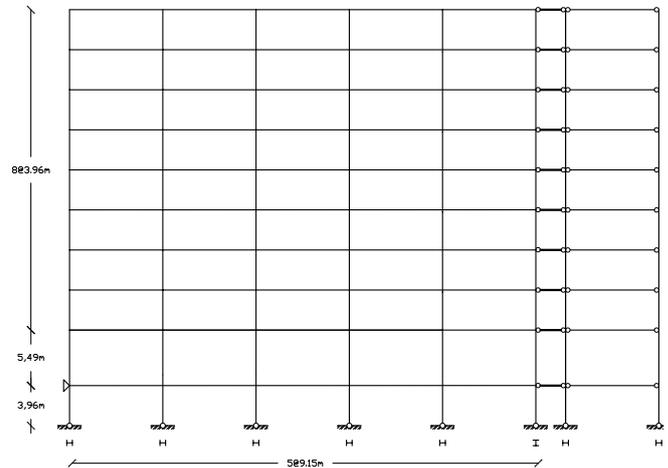
Figure 3: The LA9 steel moment-resisting frame.
