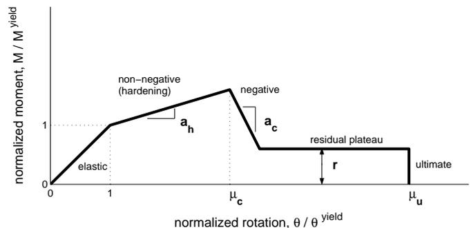
Figure 4: The moment-rotation beam-hinge backbone to be investigated and its six controlling parameters.
