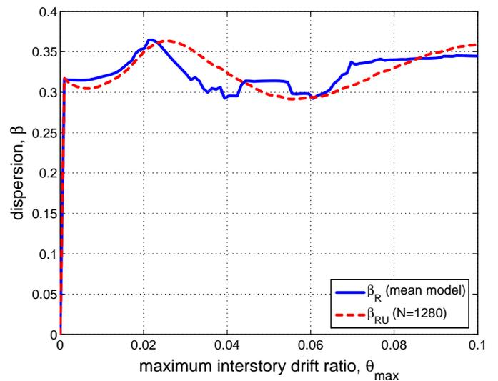
Figure 7: Comparison of dispersion of  $S_a(T_1, 5\%)$  capacity: iLHS versus the mean model.
