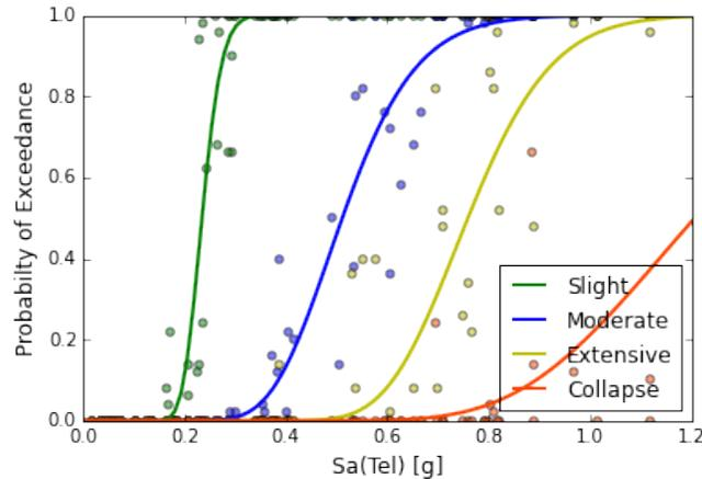
Fig. 5 – Fitting of lognormal functions considering the damage distribution from the non-linear analysis.
