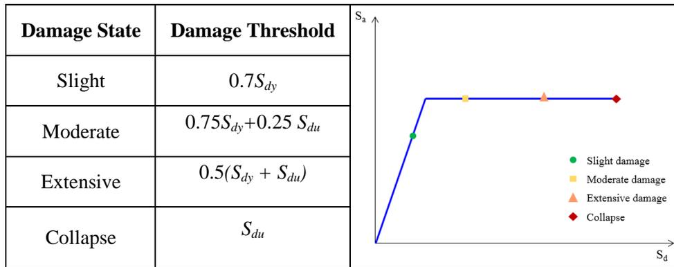
Fig. 4 - Example of a capacity-curve based damage model [14].
