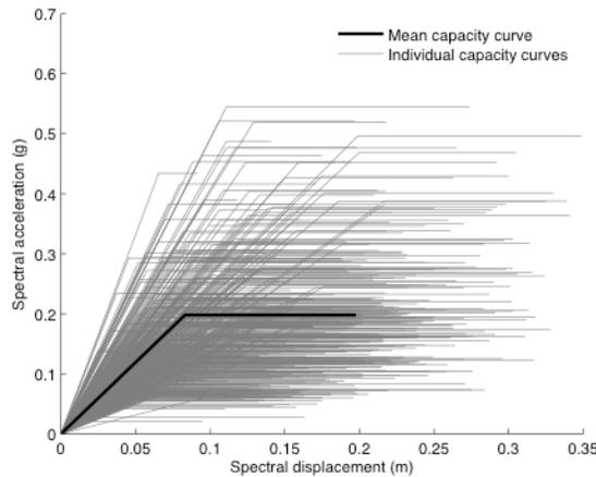
Fig. 3 - Multiple simulated bilinear elasto-plastic capacity curves
