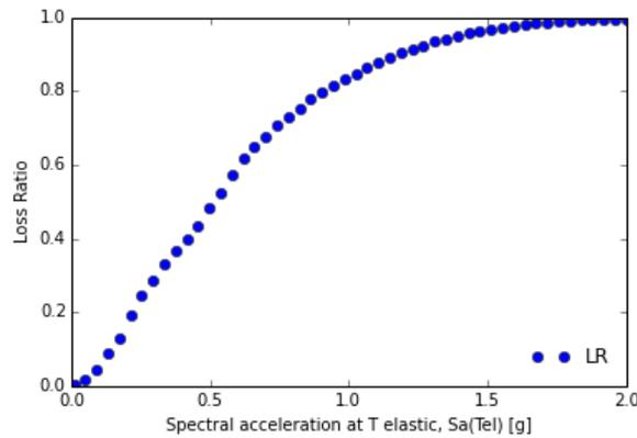
Fig. 6 – Derivation of a vulnerability function through the combination of fragility and damage-to-loss models.
