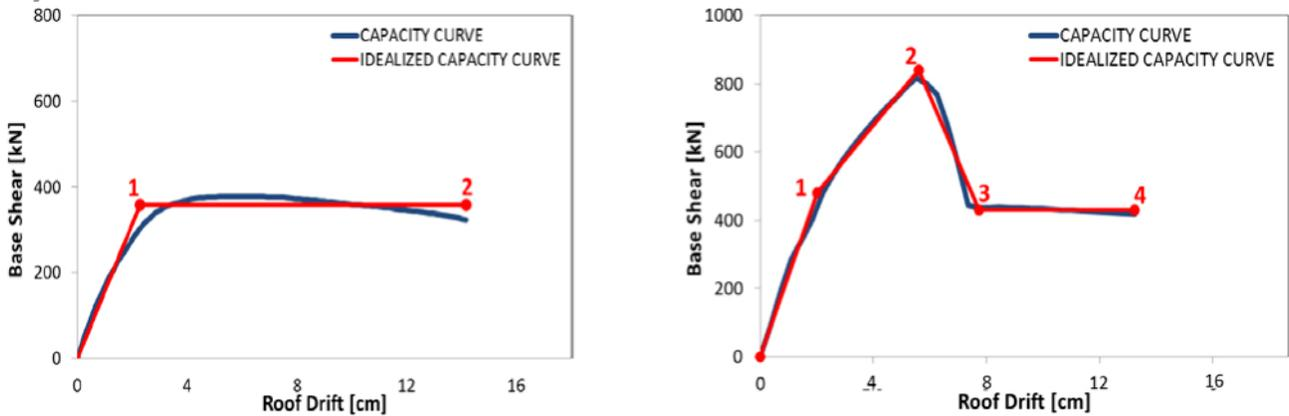
Fig. 2 - Idealized capacity curves: bilinear (L), quadrilinear (R)
