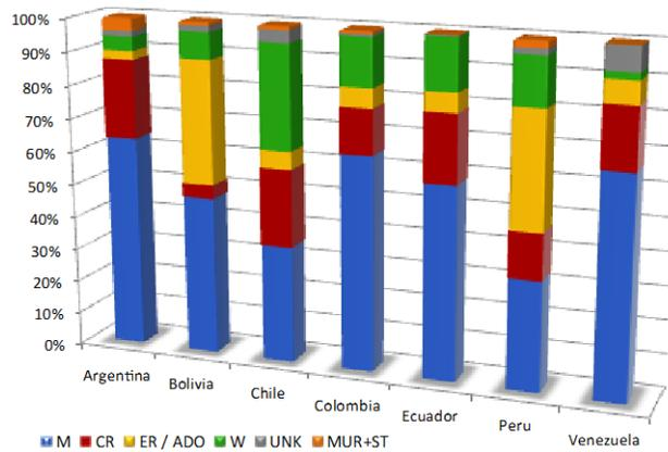
Fig. 7 – Distribution of the residential building stock according to the most common construction materials in the Andean countries [23].
