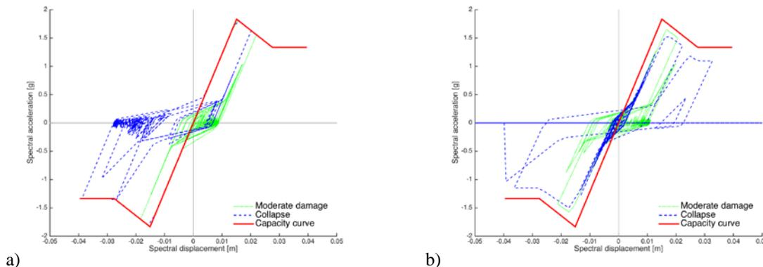
Fig. 8 – Hysteretic curves for a 2-storey confined masonry with (a) and without (b) structural degradation.
