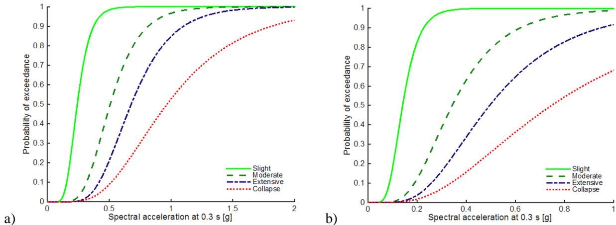
Fig. 9 – Fragility function for ductile confined masonry with two storeys (a) and adobe buildings with one storey (b).
