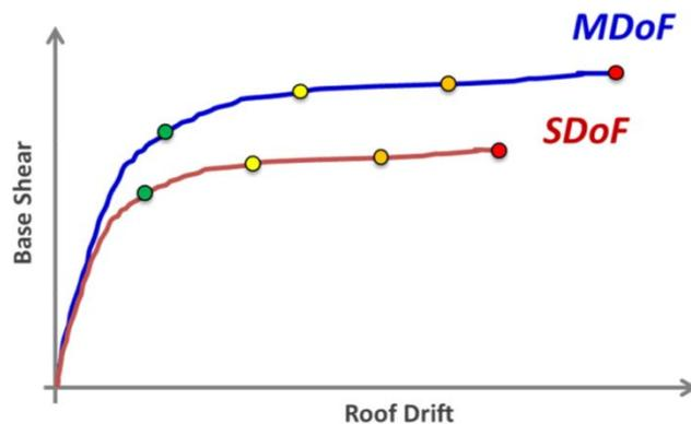
Fig. 1 - An MDOF pushover curve transformed into an equivalent SDOF curve [9].
