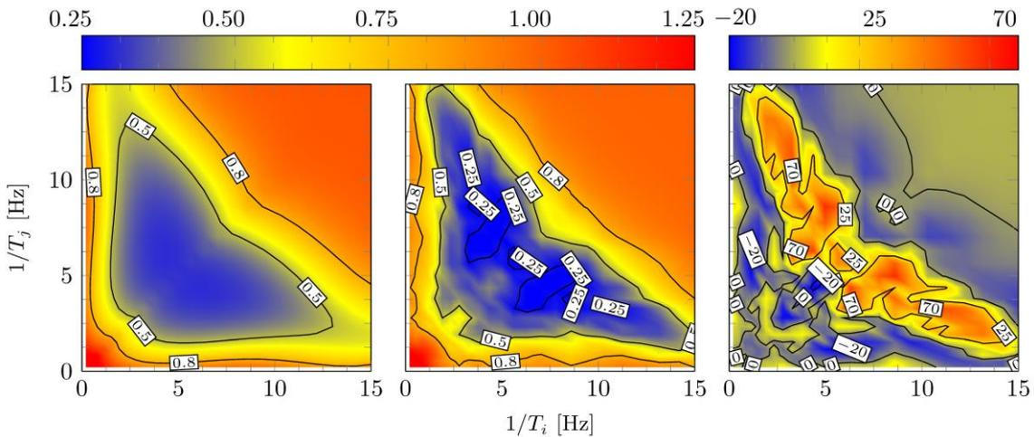
Figure 7. Cross correlation coefficients  $\rho_{ij}^*$  for the 84th percentile. Analytical approximation (left), numerical solution from optimization analysis (center), and relative error (right)
