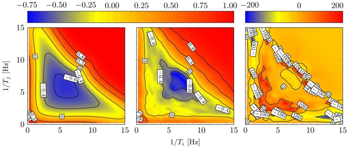
Figure 5. Cross correlation coefficients  $\rho_{ij}^*$  for the 16th percentile. Analytical approximation (left), numerical solution from optimization analysis (center), and relative error (right)
