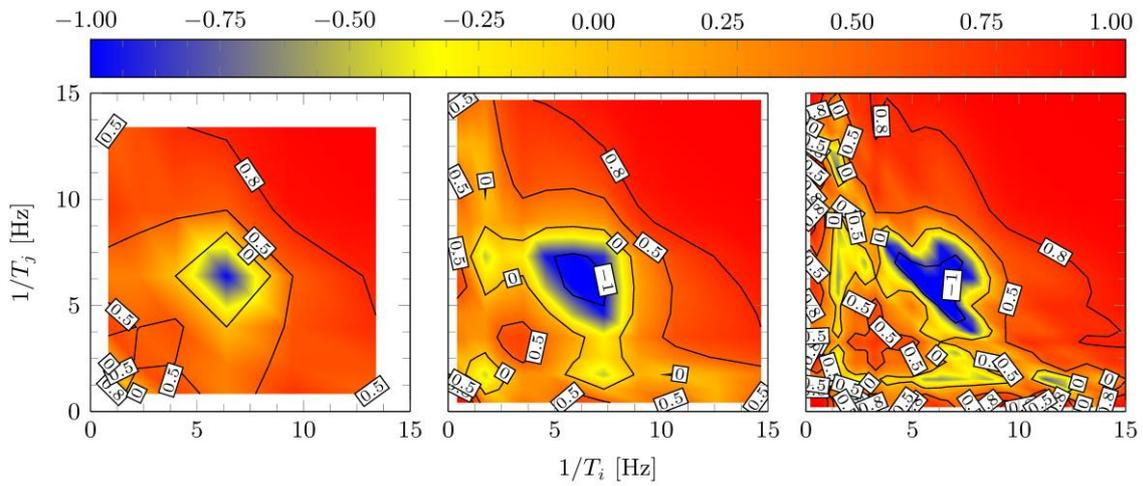
Figure 3. Cross correlation coefficients  $\rho_{ii}^*$  for 6- (left), 12- (center) and 24-story frame (right) for the Kobe earthquake record (1995, Shin – Osaka Station, NGA sequence 1116)
