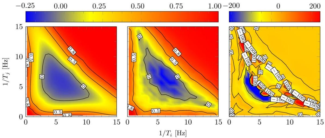
Figure 6. Cross correlation coefficients  $\rho_{ij}^*$  for the median. Analytical approximation (left), numerical solution from optimization analysis (center), and relative error (right)
