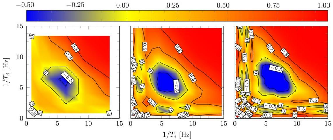
Figure 2. Cross correlation coefficients  $\rho_{ii}^*$  for 6- (left), 12- (center) and 24-story frame (right) for the Northridge earthquake record (1994, Beverly Hills – Mulhol Station, NGA sequence 953)
