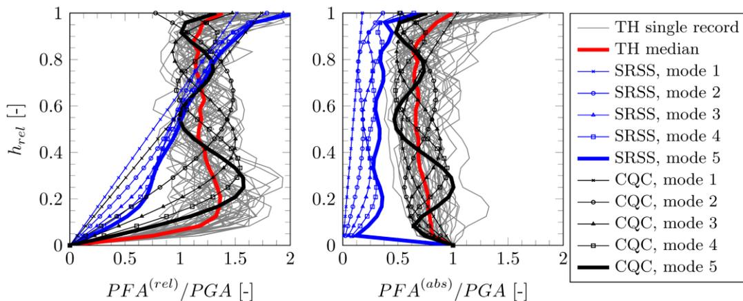
Figure 9. Profiles of normalized median peak floor acceleration demands, relative (left) and absolute (right) peak floor accelerations demands
