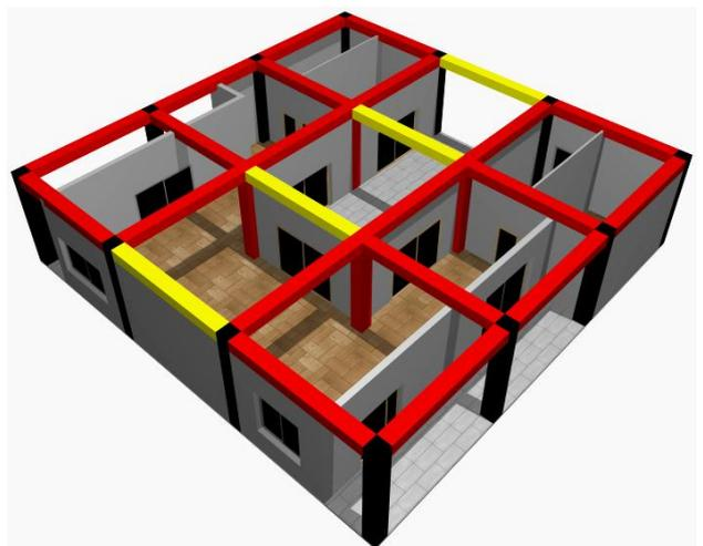
Figure 9. Ground floor 3D damage visualization at  $S_a(T_1) = 2.4g$ .
