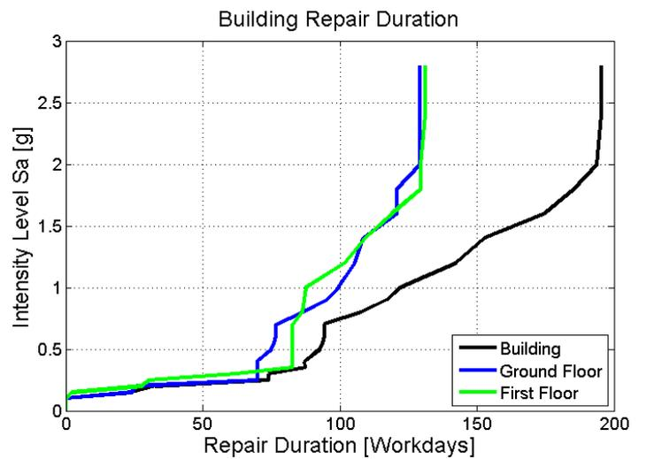
Figure 17. Building repair duration distribution per intensity level  $S_a(T_1)$ .
