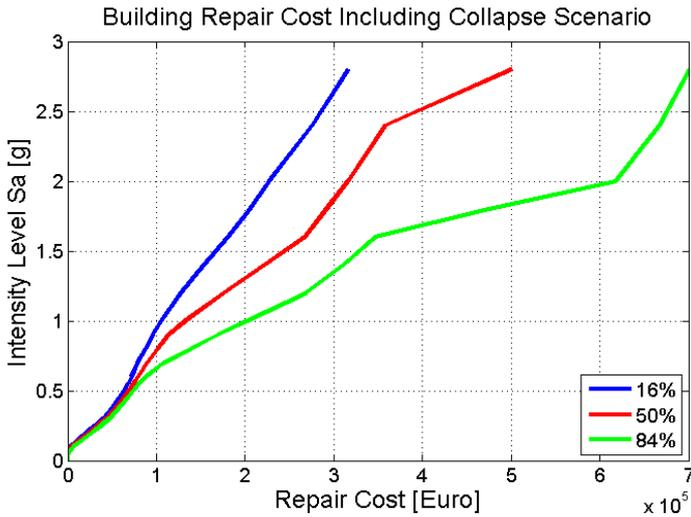
Figure 16. Building repair cost distribution per intensity level  $S_a(T_1)$ .
