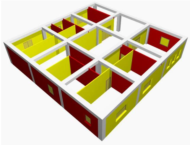
Figure 10. First floor 3D damage visualization at  $S_a(T_1) = 0.3g$ .
