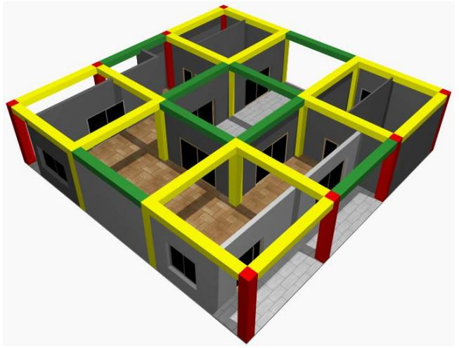
Figure 7. Ground floor 3D damage visualization at  $S_a(T_1) = 1.2g$ .
