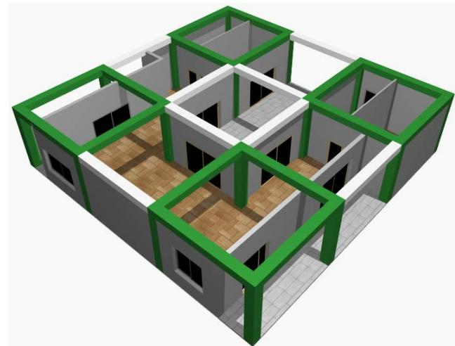
Figure 5. Ground floor 3D damage visualization at  $S_a(T_1) = 0.6g$ .
