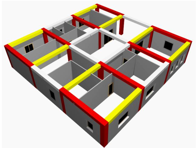
Figure 15. First floor 3D damage visualization at  $S_a(T_1) = 2.4g$ .
