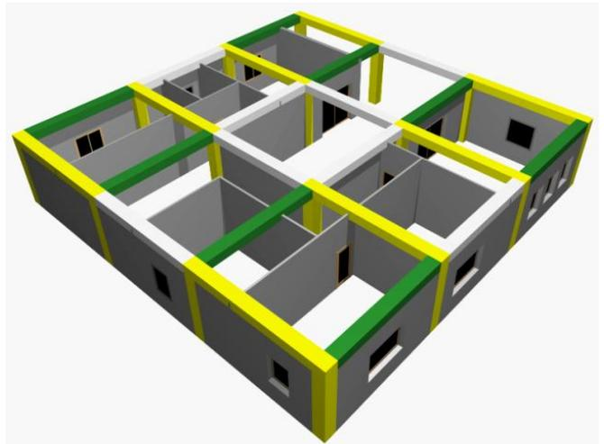
Figure 14. First floor 3D damage visualization at  $S_a(T_1) = 1.8g$ .
