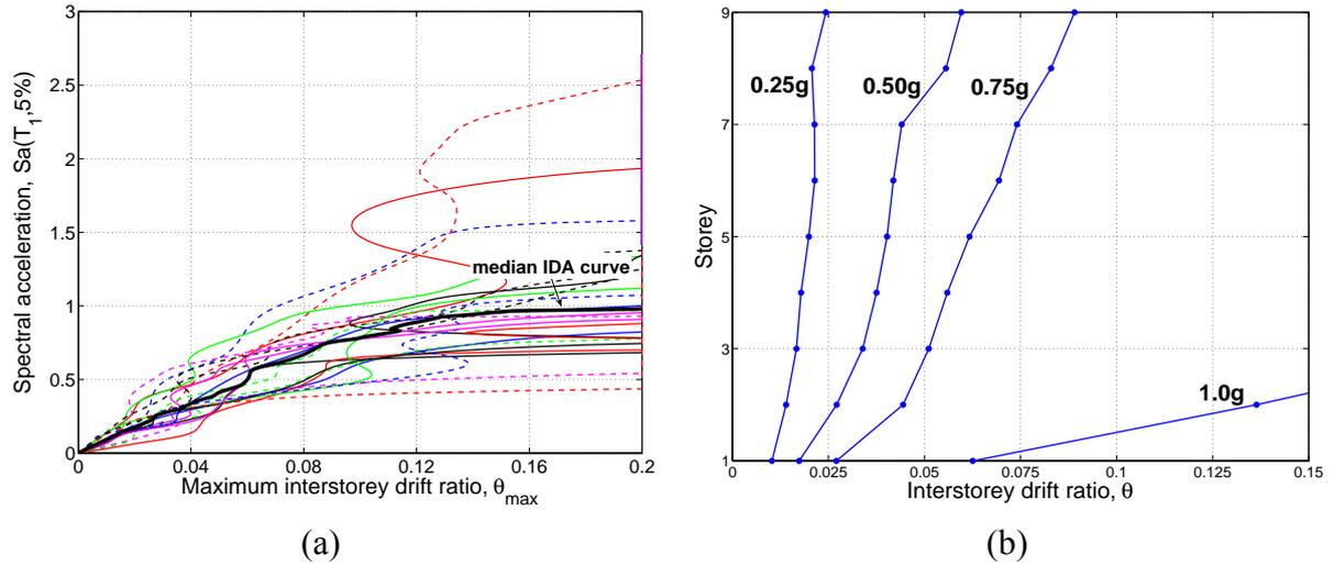
**Figure 2:** (a) Twenty IDA curves and their median curve, (b) Profiles of median interstorey demands for different  $S_a(T_1, 5\%)$  levels.
