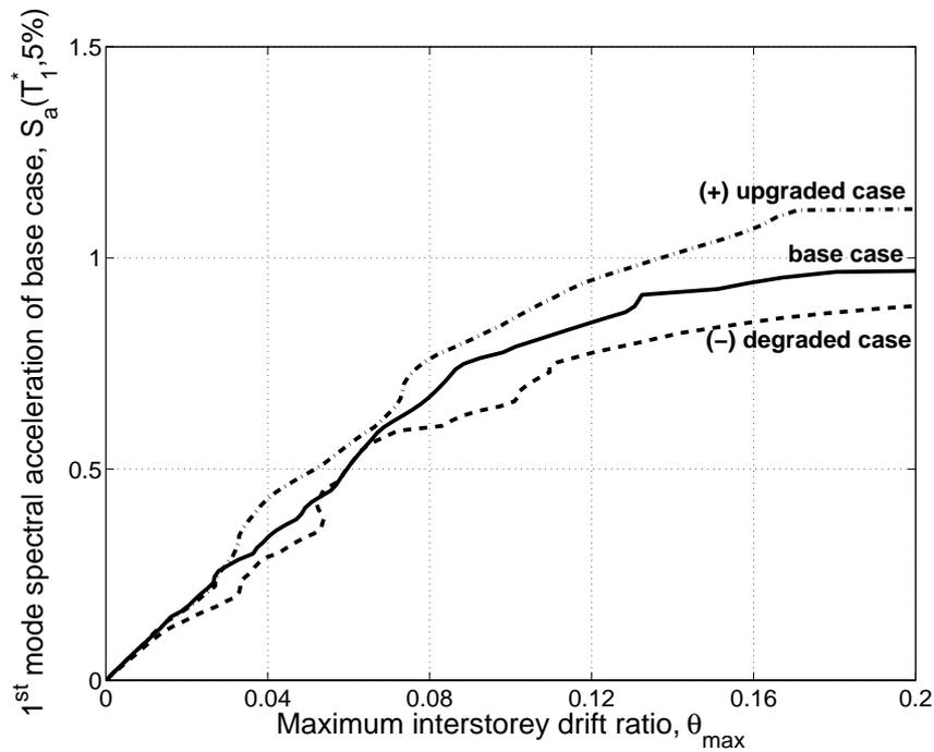
**Figure 3:** Using a common IM to compare the median IDA curve of the base case versus those produced when upgrading or degrading a structural property.
