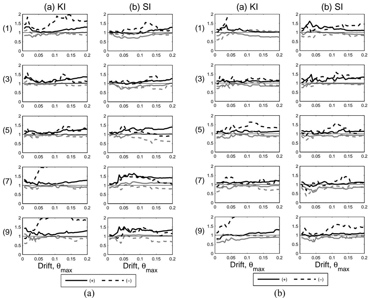
**Figure 7:** (a) Bootstrap 90% confidence intervals on the ratio of the median  $S_a(T_1^*, 5\%)$ -capacities given  $\theta_{\max}$  of the modified over the base frame, (b) Bootstrap 90% confidence intervals on the ratio of the dispersion of  $S_a(T_1^*, 5\%)$ -capacities given  $\theta_{\max}$  of the modified over the base frame. Light-coloured lines are used for the lower bound and darker ones for the upper bound.
