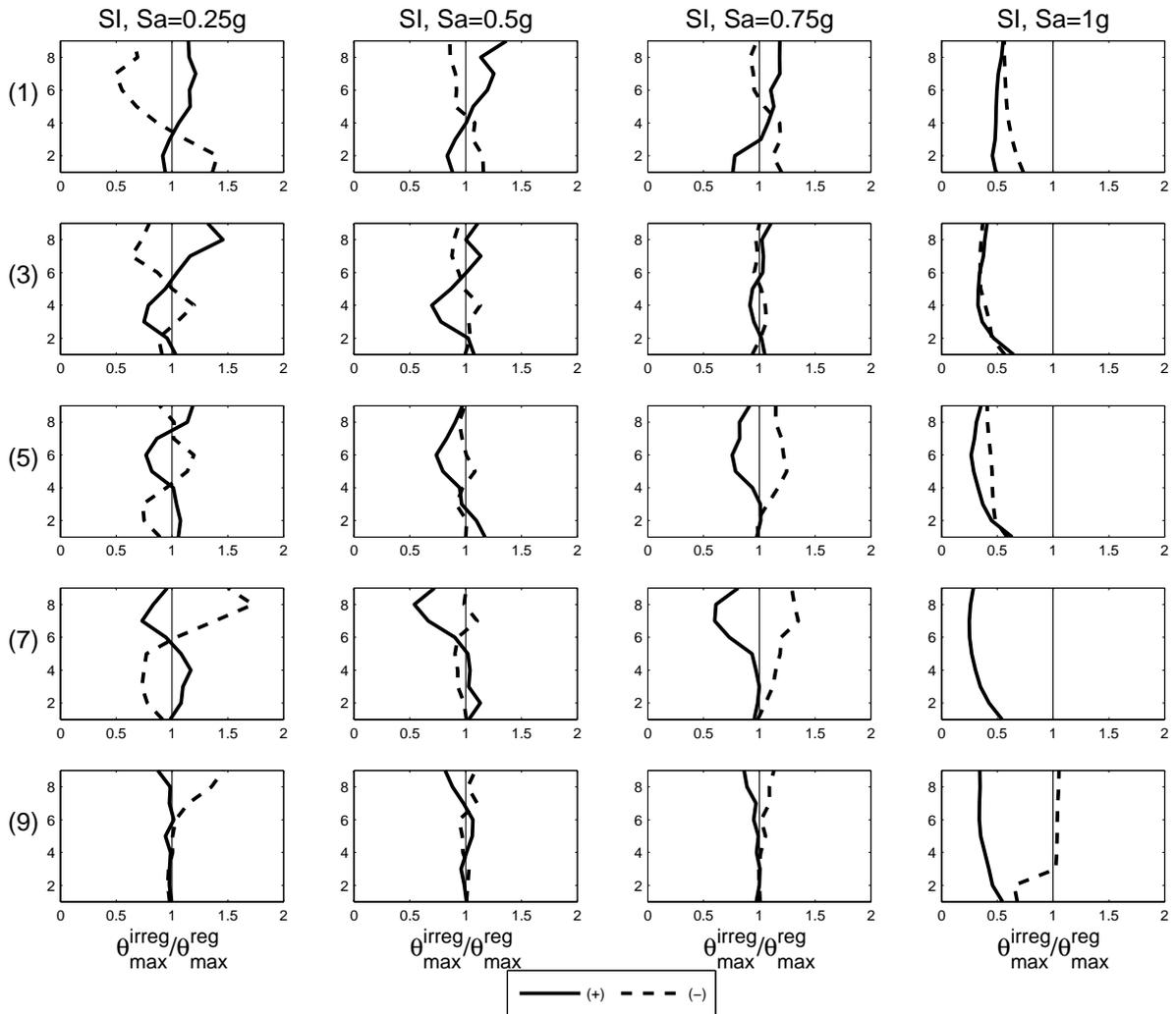
**Figure 6:** Normalized median interstorey drift demands for single-storey strength irregular (SI) cases for four  $S_a(T_1^*, 5\%)$ -levels.
