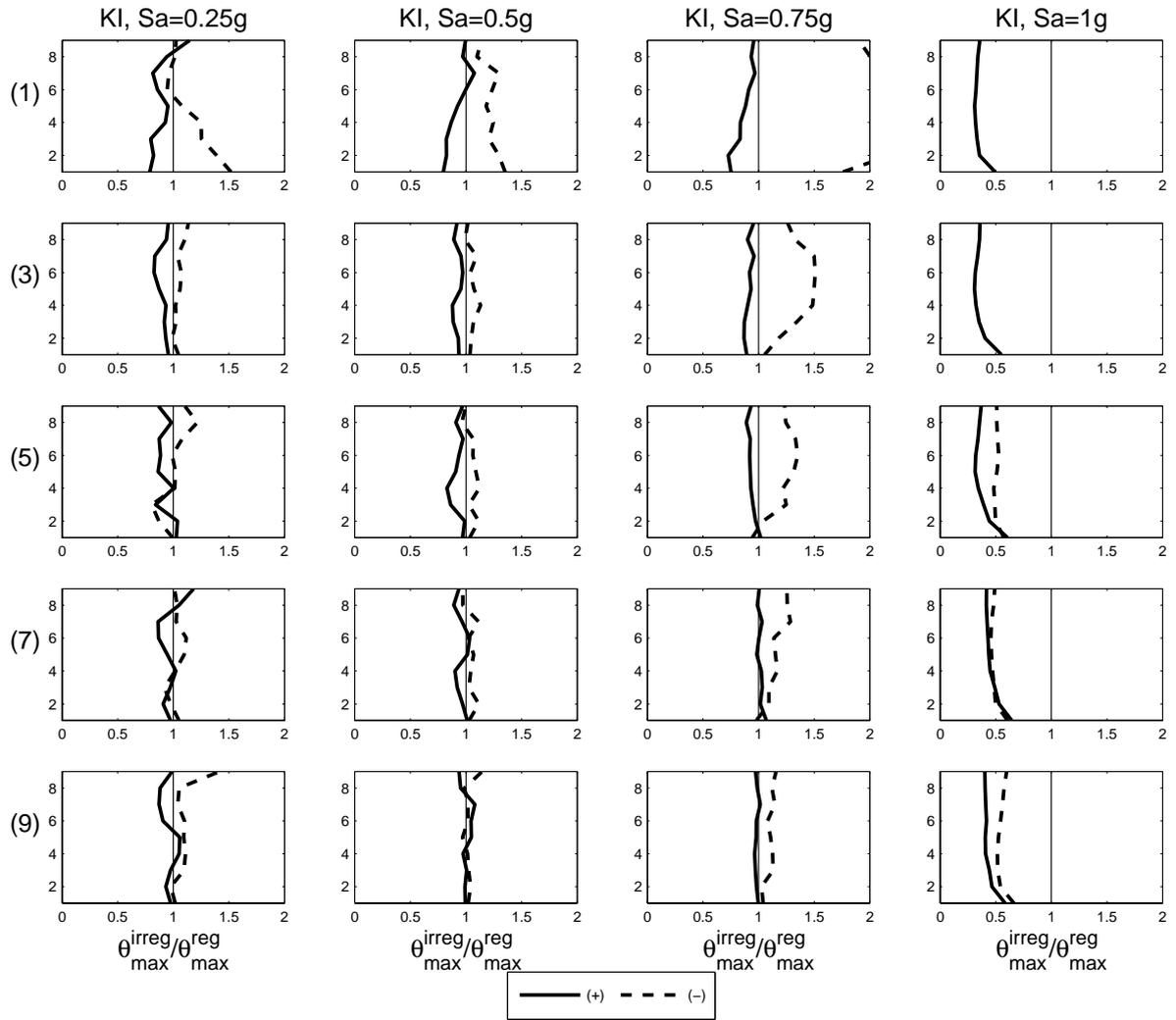
**Figure 5:** Normalized median interstorey drift demands for single-storey stiffness irregular (KI) cases for four  $S_a(T_1^*, 5\%)$ -levels.
