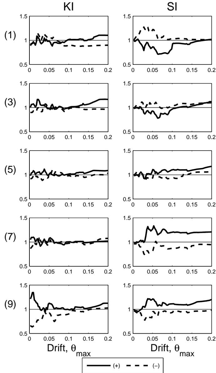
**Figure 4:** The median  $S_a(T_1^*, 5\%) - \theta_{max}$  capacities for the upgraded and the degraded cases, normalized by the corresponding base case values.
