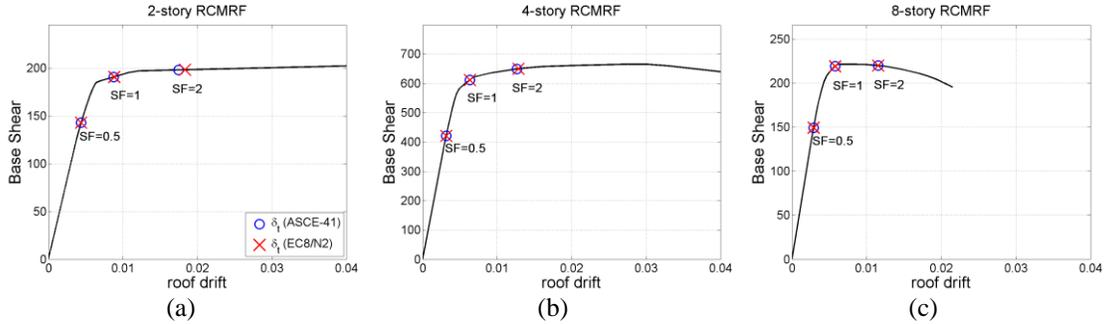
Figure 4. First mode static pushover curves and target displacement estimates for the 2-, 4-, and 8-story reinforced concrete moment frames, for ground motion scale factors of 0.5, 1.0, and 2.0.
