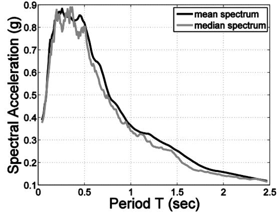
Figure 2. 5%-damped unscaled mean and median response spectra of the 44 ground motion records used in this study.
