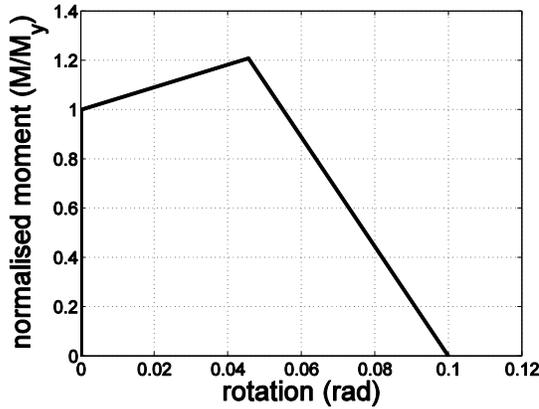
Figure 1. Typical moment-rotation relationship used for the plastic hinge part of component models.
