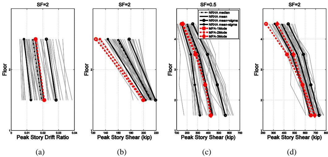
Figure 8. Estimates made with modal pushover analysis and profiles of (a) story drifts and (b) story shears for the 2-story RCMRF at SF=2, and profiles of story shears for the 4-story RCMRF at (c) SF=0.5 and (d) SF=2.
