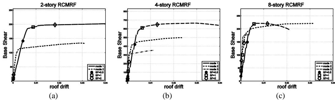
Figure 7. Static pushover curves and target displacement estimates for the 2-, 4-, and 8-story reinforced concrete moment frames, for ground motion scale factors of 0.5, 1.0, and 2.0.
