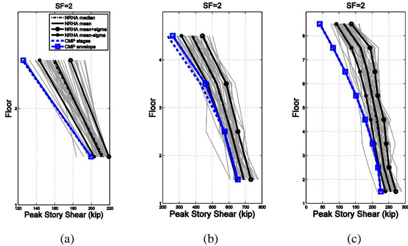
Figure 10. Story shear estimates using consecutive modal pushover analysis for the 2-, 4-, and 8-story reinforced concrete moment resisting frame
