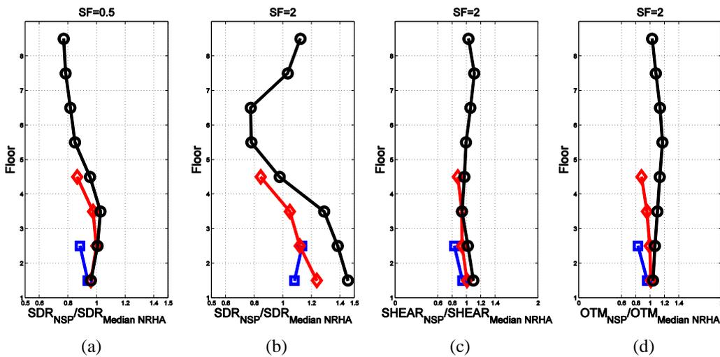
Figure 9. Ratio of modal pushover analysis results and nonlinear response history analysis results for the reinforced concrete moment resisting frames: (a) peak story drift (SF=0.5), (b) peak story drift (SF=2.0), (c) peak story shears (SF=2.0), and (c) peak overturning moments (SF=2.0).
