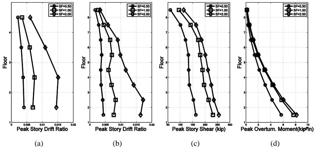
Figure 3. Profiles of median peak response quantities for SF=0.5, 1.0, and 2.0: (a) story drifts for the 4-story RCMRF, and (b) story drifts, (c) story shears, and (d) overturning moments for the 8-story RCMRF.
