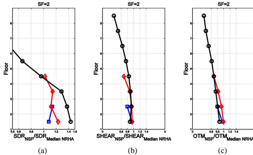
Figure 11. Ratio of Consecutive Modal Pushover Analysis results to NRHA results for the reinforced concrete moment resisting frames, for SF=2: (a) peak story drifts, (b) peak story shears, and (c) peak overturning moments.
