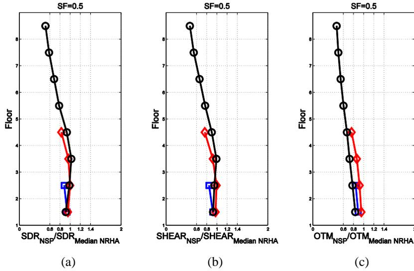
Figure 5. Ratios of first mode NSP and NRHA response estimates for SF=0.5: (a) peak story drifts, (b) peak story shears, and (c) peak overturning moments.
