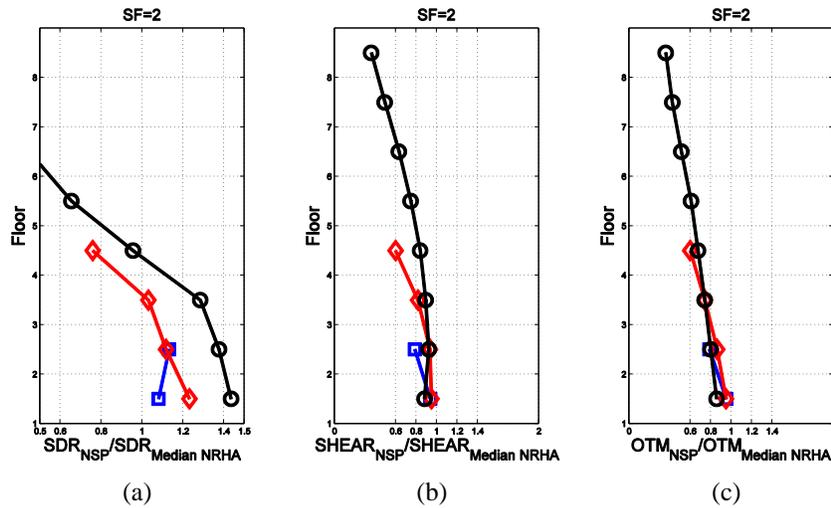
Figure 6. Ratios of first mode NSP and NRHA response estimates for SF=2.0: (a) peak story drifts, (b) peak story shears, and (c) peak overturning moments.
