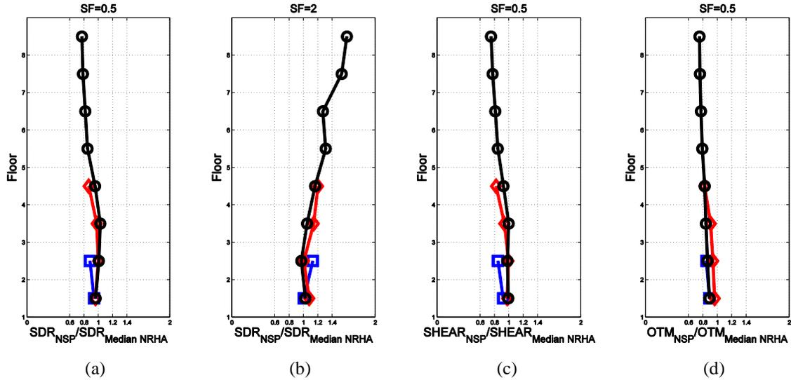
Figure 12. Ratio of elastic Modal Response Spectrum Analysis results to NRHA results for the reinforced concrete moment resisting frames, for SF=0.5: (a) peak story drifts, (b) peak story shears, and (c) peak overturning moments.
