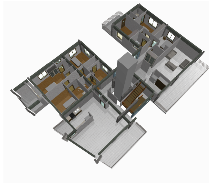
Figure 2. 3D BIM of case-study building floor with structural, non-structural components contents in undamaged state.
