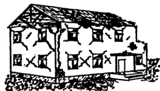
GRADE 4: Very heavy damage
