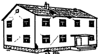
GRADE 2: Moderate damage
