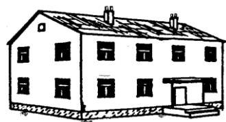
GRADE 1: Negligible to slight damage
