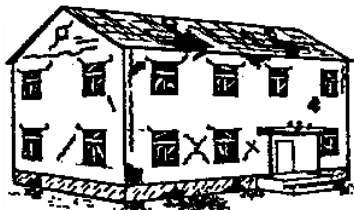
GRADE 3: Substantial to heavy damage
