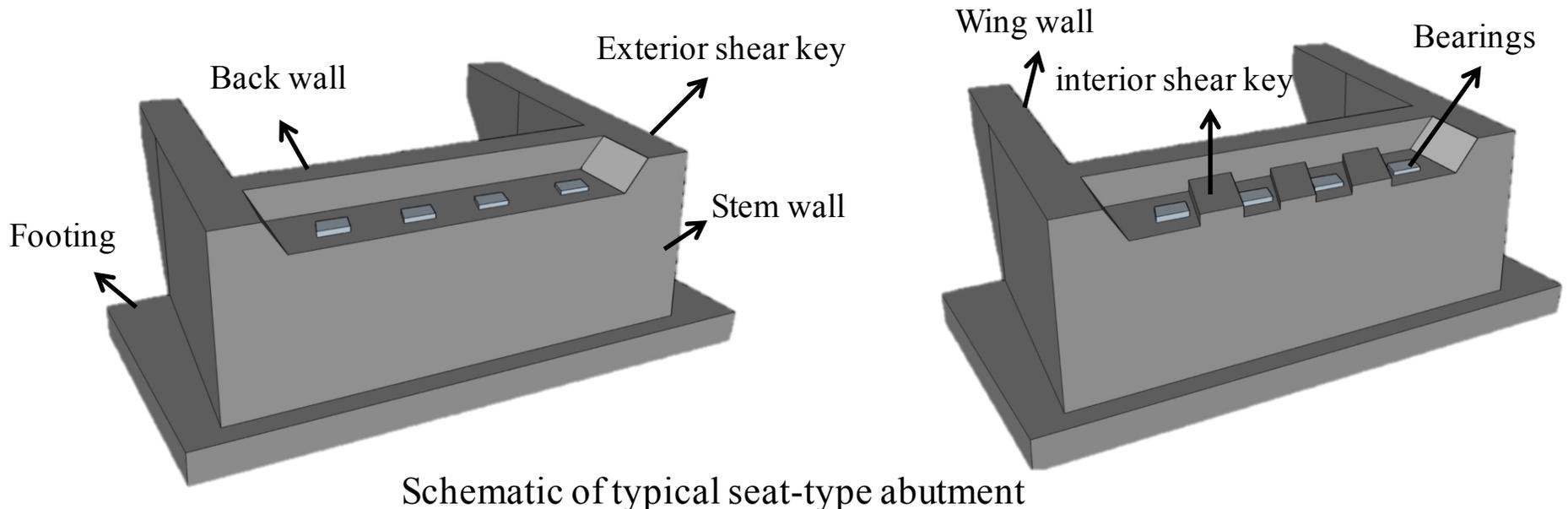
Schematic of typical seat-type abutment
