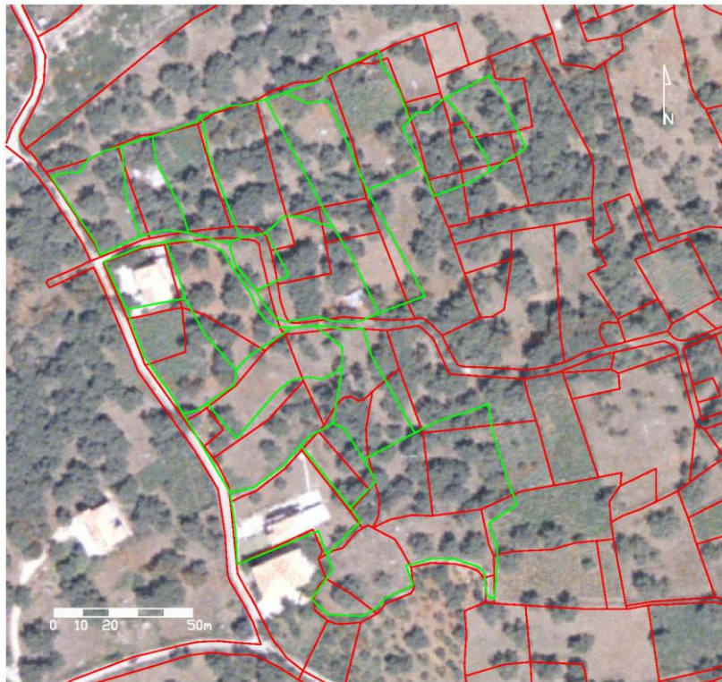
Figure 2: Cadastral survey produced by the contractor (in red); cadastral survey produced by KT (in green)
