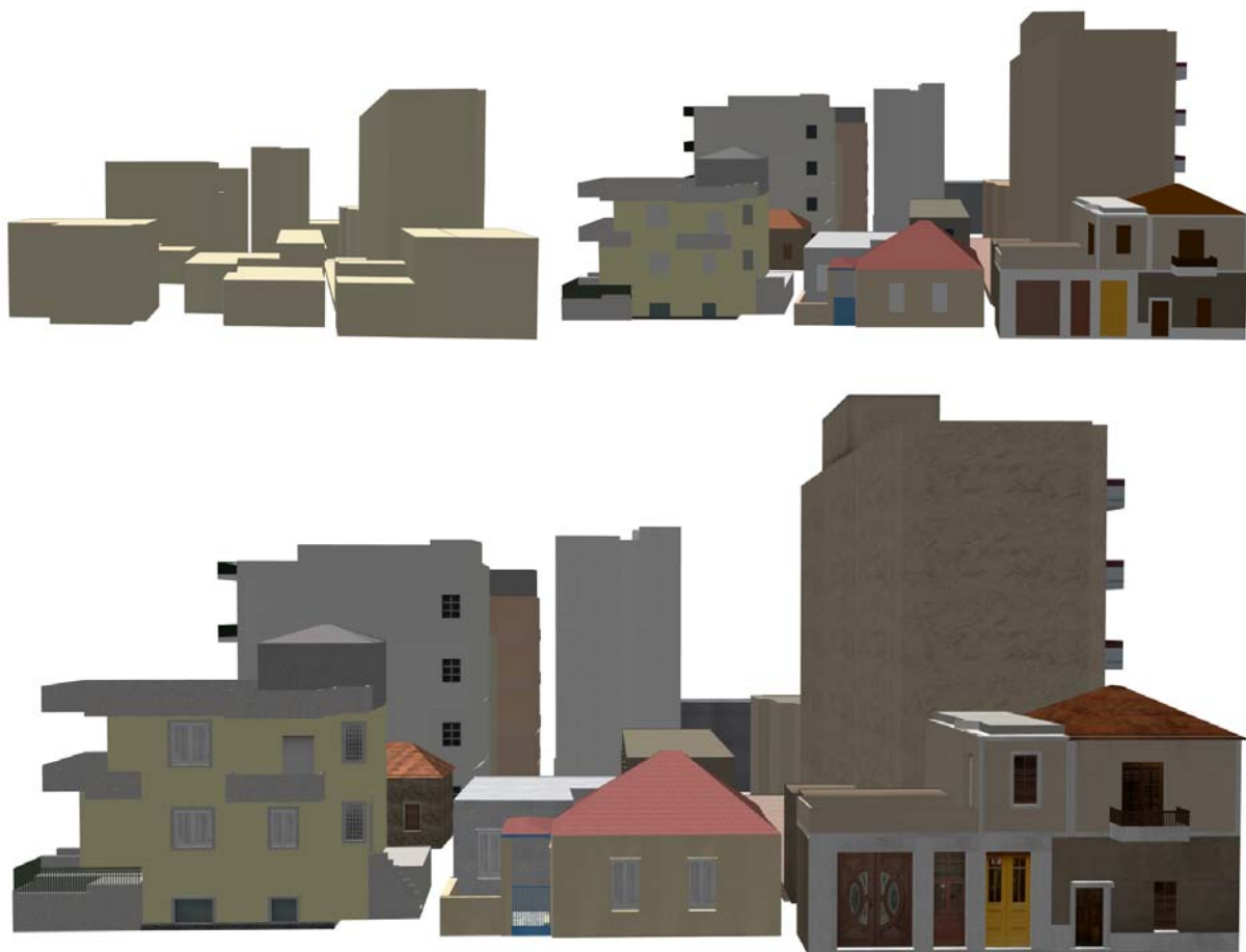
Figure 4. 3D views of the building models at LoD1 (top-left), LoD2 (top-right) and LoD3 (bottom)
