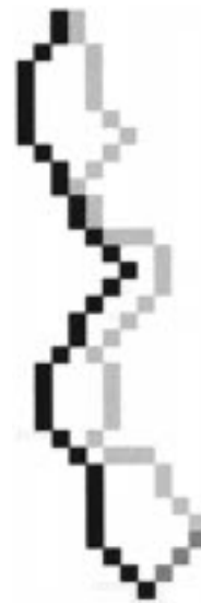
Fig. 6. Depiction of “fixed” and rotating chain belonging to two different frescos (pieces). Black pixels belong to the “fixed” chain. Light gray pixels belong to the “rotating” chain. Darker gray pixels bridge the last pixel of the two chains (“barrier” line). Notice that the “rotating” (light gray) chain ends when it intersects the “barrier” line.
