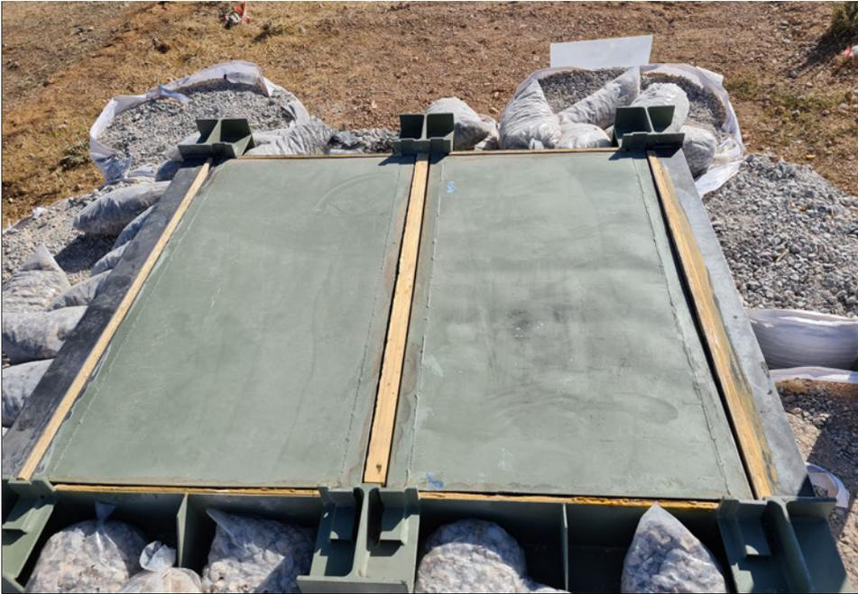
Figure 6-10: Photo of the specimens after the explosion
