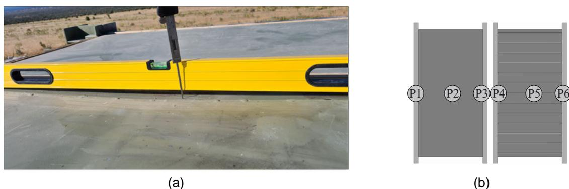
Figure 6-12: Permanent deflections after the explosion: (a) Visual representation of the deflection of the central girt of the panel with stiffeners; (b) Points of interest in plan for the determination of maximum and permanent displacement (solid plate - left, panel with stiffeners - right)
