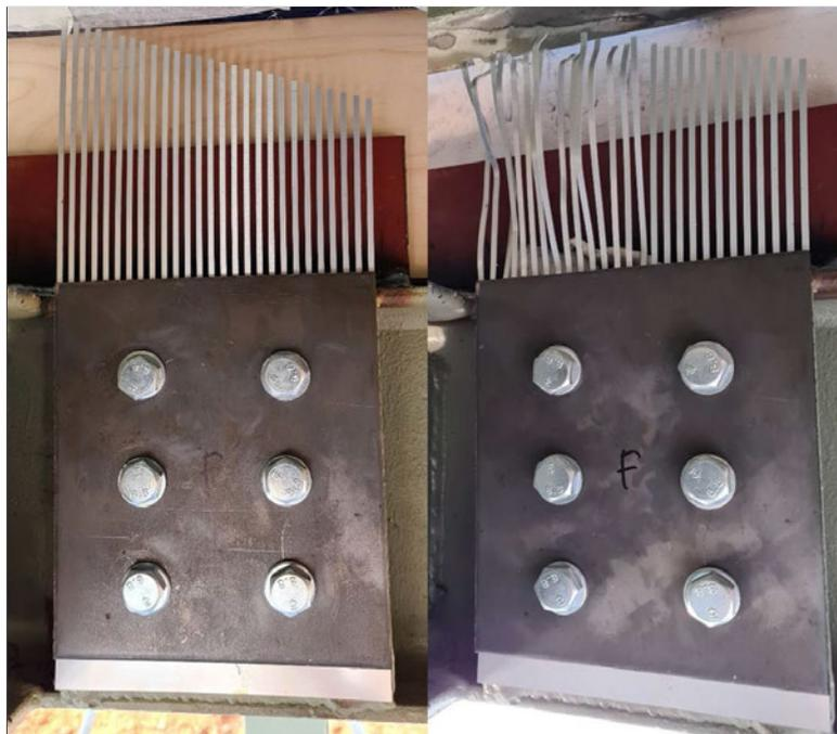
Figure 6-11: Displacement device, before and after the explosion
