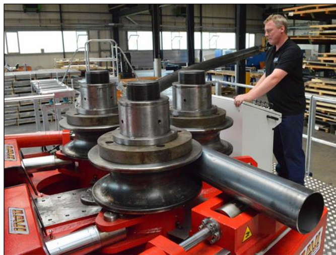
Figure 6-1: Example of roller-bending a CHS workpiece.
