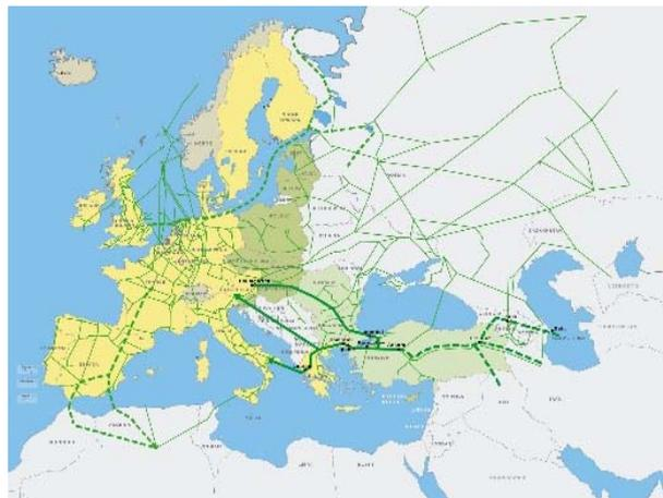
Figure 1-1: Existing and new natural gas transmission pipeline network of Europe ("European Commission, Energy - Infrastructure" 2008)
