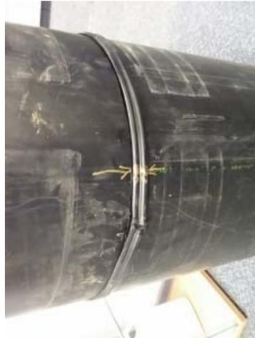
Figure 1-9: Pipe girth weld tensile fracture ("Impact Solutions" 2016)
