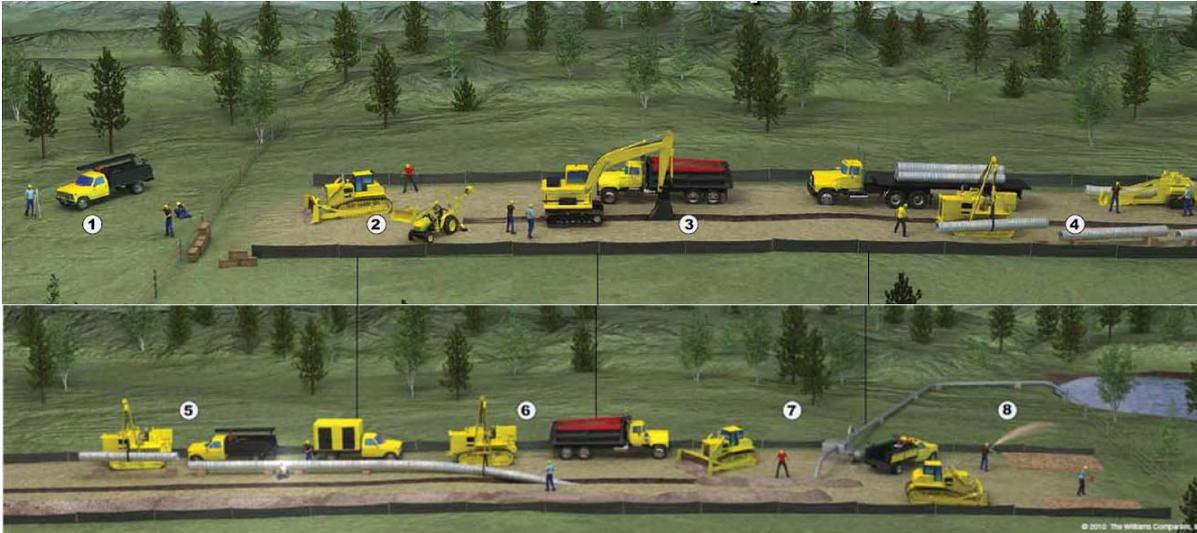
Figure 1-5: Stages of onshore buried pipeline construction (Constitution Pipeline 2016)
