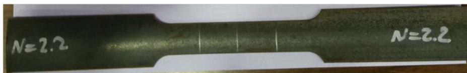
Figure 3-11: Typical tensile coupon
