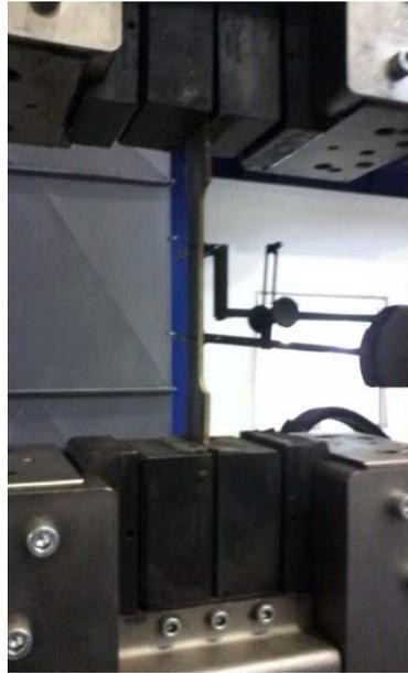
Figure 3-12: Coupon during tensile test
