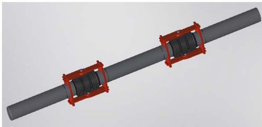
Figure 1-13: Schematic illustration of the introduction of flexible joints in a pipe
