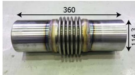
Figure 3-17: Flexible joint (single bellow-type) used in the experimental investigation
