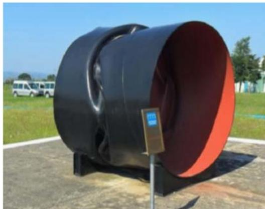
Figure 1-10: Wrinkling of a 2.2m diameter steel water pipe at a fault crossing in Kullar, Izmit in the 1999 Kocaeli Earthquake (Uckan et al. 2015)
