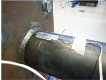
Figure 3-10: Strain gauge (SG) placed on specimen crown
