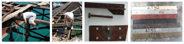
Preparation of specimens and tension tests for evaluation of mechanical characteristics
