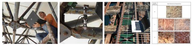
On-site hardness measurements for approximate evaluation of mechanical characteristics
