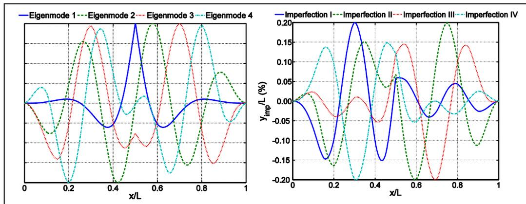
Figure 2: Eigenmode shapes (left) and imperfection shapes (right).
