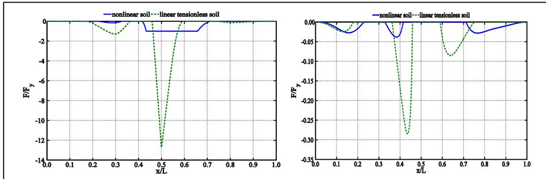
Figure 5: Upward (left) and downward (right) soil spring force for nonlinear vs. elastic tensionless soil.
