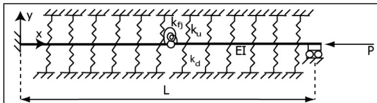
Figure 1: Fixed-fixed beam with flexible joint resting in deformable foundation under compressive load.
