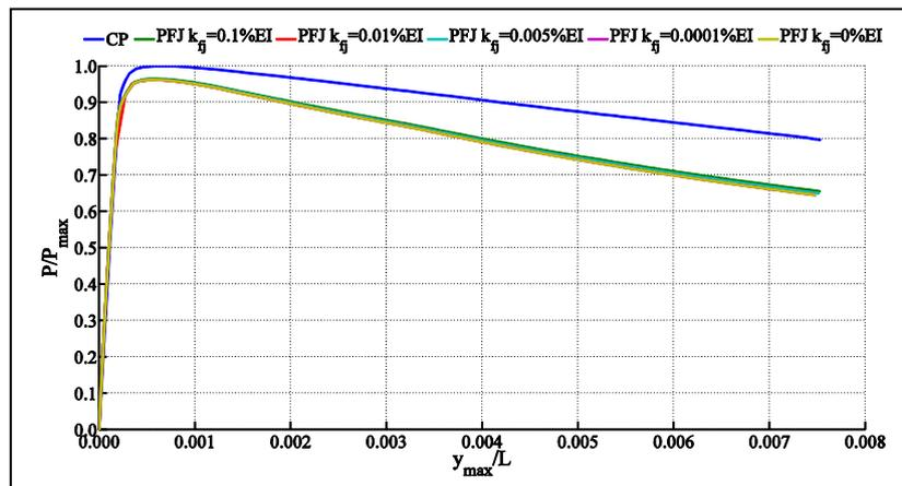
Figure 6: Comparison of equilibrium paths of continuous pipeline and pipelines with flexible joint.
