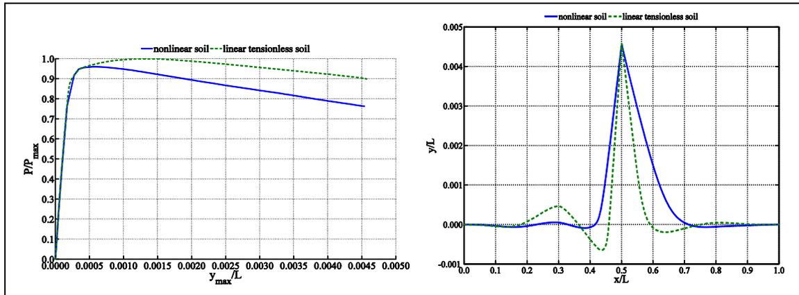
Figure 4: Equilibrium path (left) and deformed shape (right) for comparison of nonlinear vs. elastic tensionless soil cases.
