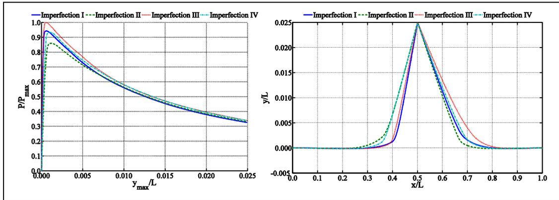
Figure 3: Equilibrium path (left) and deformed shape (right) for all imperfection cases.
