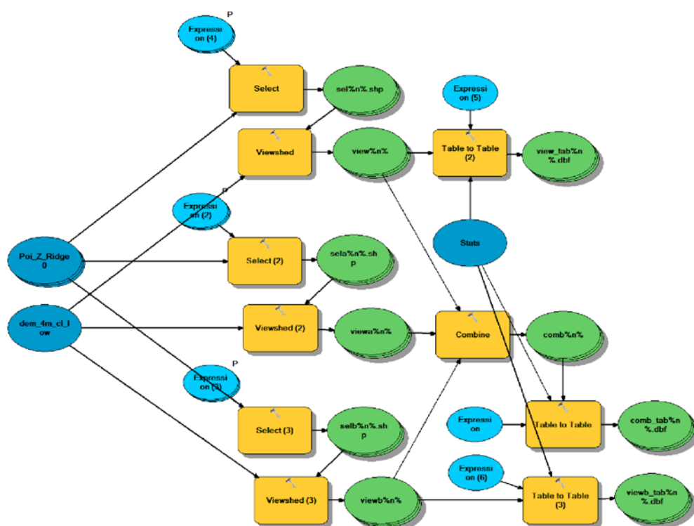
Figure 8: Model utilized to automate the workflow of the generation of i) multiple viewsheds and their numeric elements and ii) combined viewsheds and their numeric elements.
