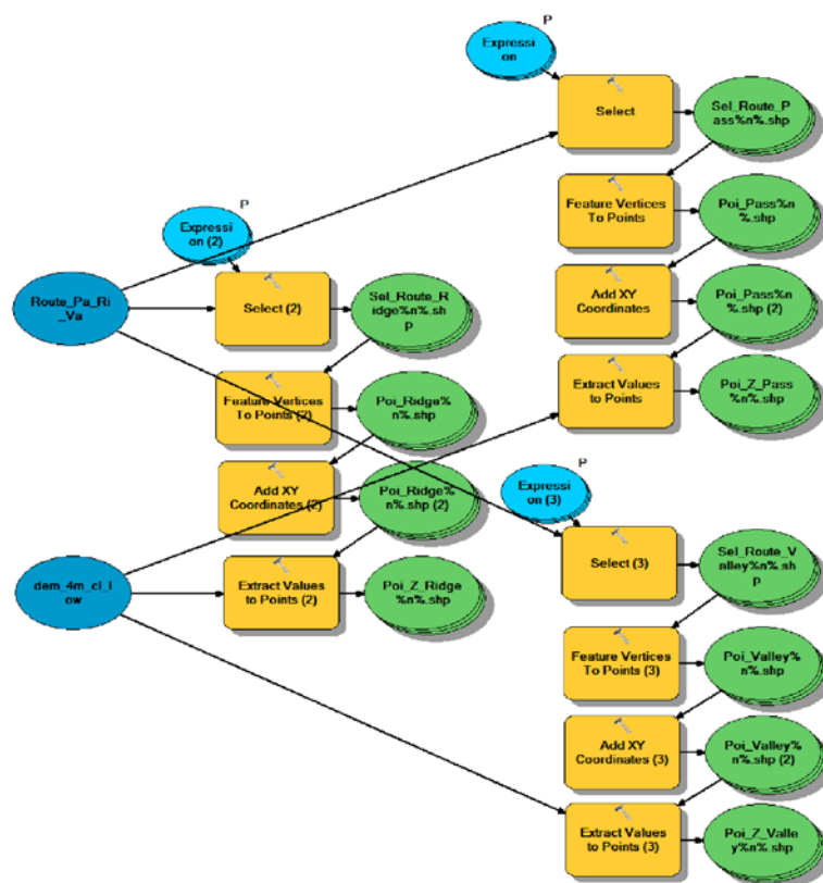
Figure 5: Workflow model of the conversion of the initial polyline feature class maintaining all the topographic feature routes into nine (9) separate point feature classes (shapefile layers) with XYZ coordinates.
