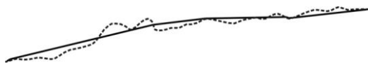
Figure 5: An example of generalization of a \epsilon -part of Type D (Initial line: dotted and generalized line: solid).
