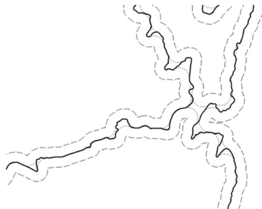
Figure 2. An example of Perkal's rolling disc method implemented in computer environment.
