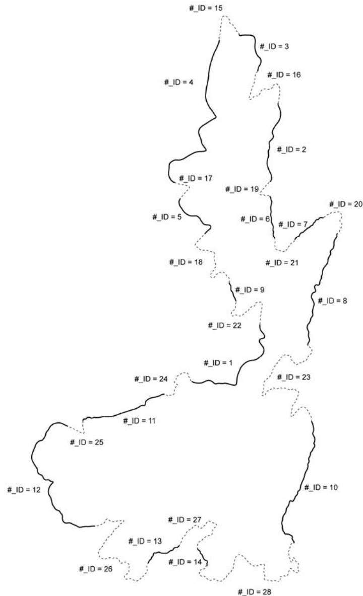
Figure 4. An example of a coastline segmented into parts by applying the rolling disc method of Perkal.
