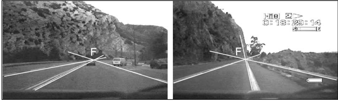
Figure 4. Graphical determination of vanishing points.
