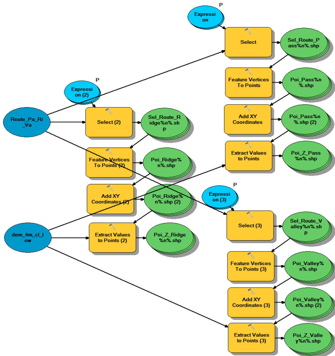
Figure 55: Workflow model of the conversion of the initial polyline feature class maintaining all the topographic feature routes into nine (9) separate point feature classes (shapefile layers) with XYZ coordinates.
